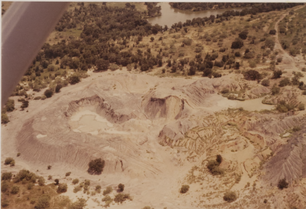
Figure 25. Oblique aerial photograph of small ponds on the surface of a spoil mound at mine-site number PP/G-2-51, Palo Pinto County, Texas, 1979. Mound is unstable and ponds may drain suddenly if retaining slopes fail. Photograph by William Hupp, Texas Department of Water Resources (used with permission).
