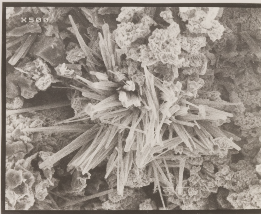
Figure 24. Scanning-electron micrograph of melanterite (?), \text{FeSO}_4 \cdot 7\text{H}_2\text{O} , monoclinic, a product of the oxidation and hydration of marcasite under atmospheric conditions. Magnification is x 5000, not x 500 as shown. Leftmost increment in bar scale is 1 micron in length. Melanterite tentatively identified by D. S. Barker, Department of Geological Sciences, The University of Texas at Austin.
