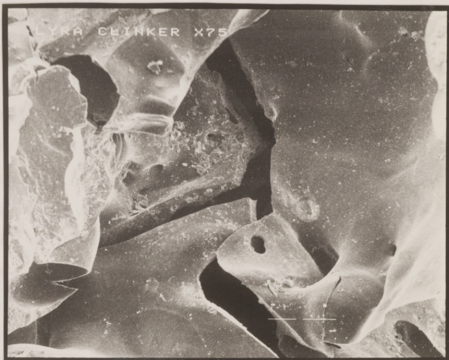
Figure 18. Scanning-electron micrograph of completely fused shale from spoil mound at mine-site number PP/G-2-9, Palo Pinto County, Texas. Viscously fused shale. Central part of fig. 17, magnified to x 75. Leftmost increment in the bar scale is one micron in length. Fractures formed when melt-liquid chilled and solidified as bubbles of gas were contracting owing to the reduction in temperature. Surfaces on opposite sides of fractures are in different planes.
