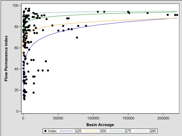
Figure 10: Quantile regression of Flow Permanence Index by drainage area of each EII reach
