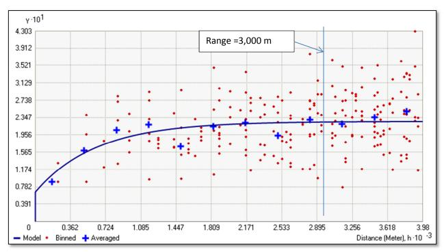
Figure 5: Semivariogram Using Indicator Kriging with a Threshold of 0.85.
