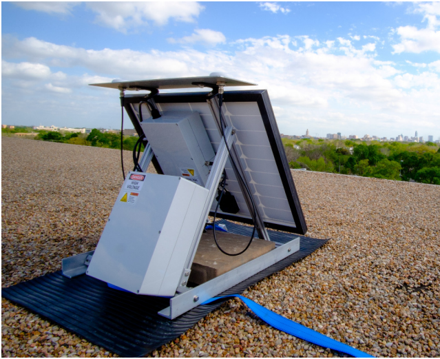
Fig. 15. A low-cost reference station in the University of Texas at Austin reference network, deployed in March, 2016, in Austin, Texas.
