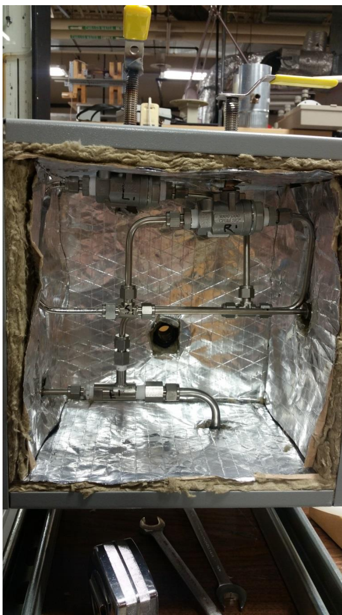
Figure A.6: Stream switching box interior. Eductor is located at the bottom of the box. Waste stream from the eductor exits at the bottom of the box. Sample exit to the right. The two sample inlets are behind the valves at the top of the box.
