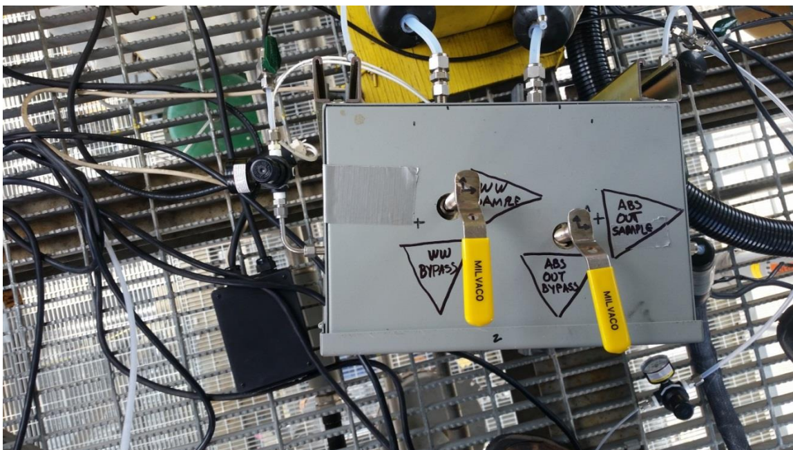
Figure A.8: Switching box in the field. Sampling and bypass instructions are on the top of the box: user places the valve handle over the selected operation.
