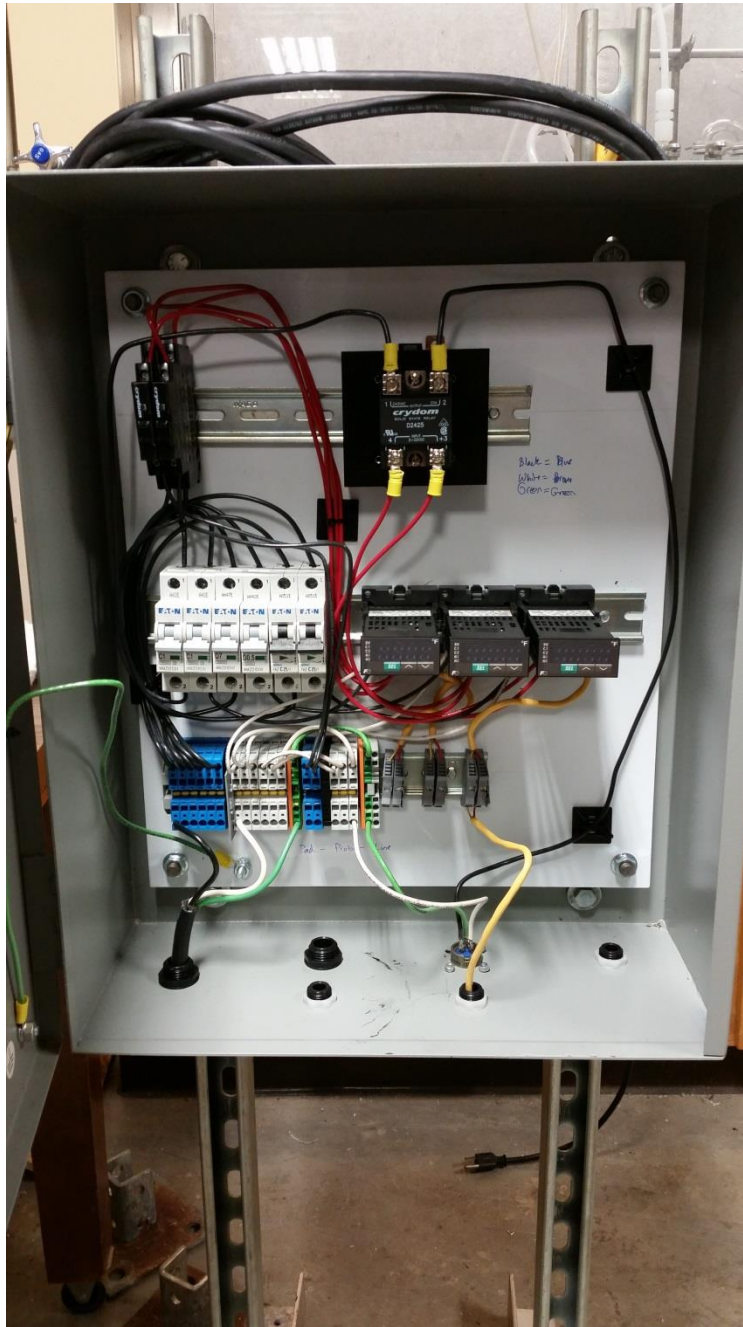
Figure 2.8: Electrical temperature control box for heated sampling equipment.
