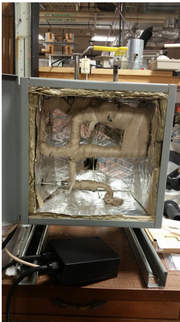
Figure A.7: Switching boxes with heat tape and wiring. Heat tape and thermocouple wiring enters the rear of the box through grip-cord connections. Sample selection valves are visible at the top of the box (yellow handles).
