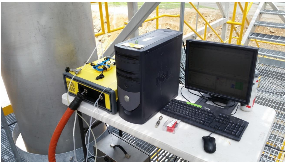
Figure A.9: DX-4000 analyzer setup. The FTIR analyzer is yellow box on the left side. CPU and user interface are adjacent on top of the table. The sample pump and filter unit is the metal box below the analyzer.
