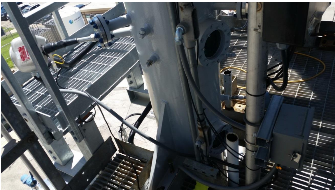
Figure 5.5: FTIR probe (to the left) for sample extraction between second and third stages of packing at UT-SRP pilot plant.
