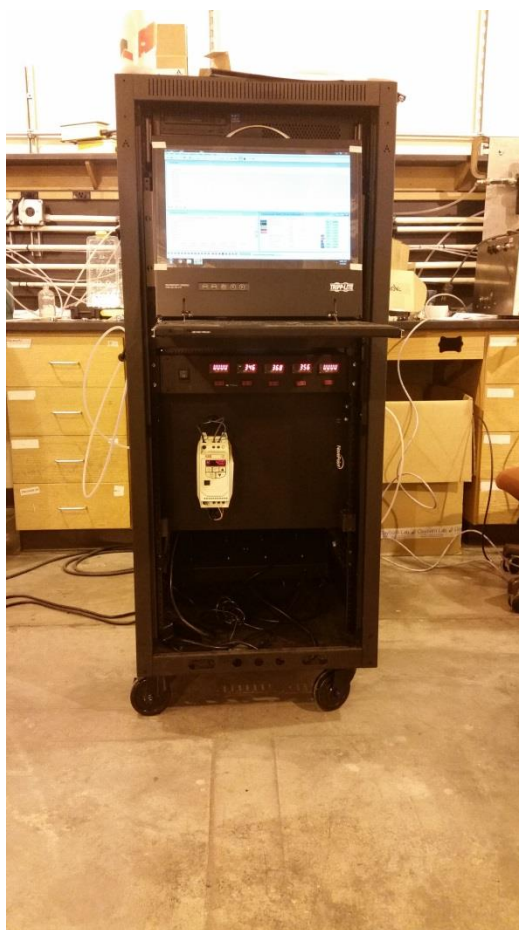
Figure C.1: Gasmet™ CX-4000 FTIR in server rack
