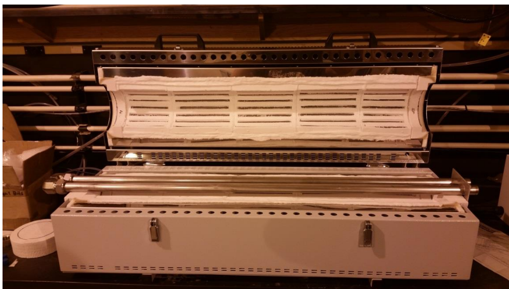
Figure 3.4: Carbolite HST 12/900 furnace with two-pass catalyst bed
