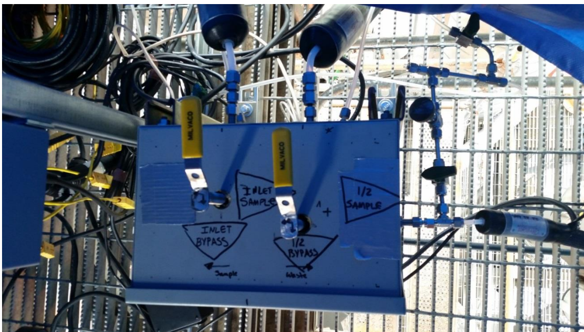
Figure A.13: Sample switching box with N 2 background adaptation.
