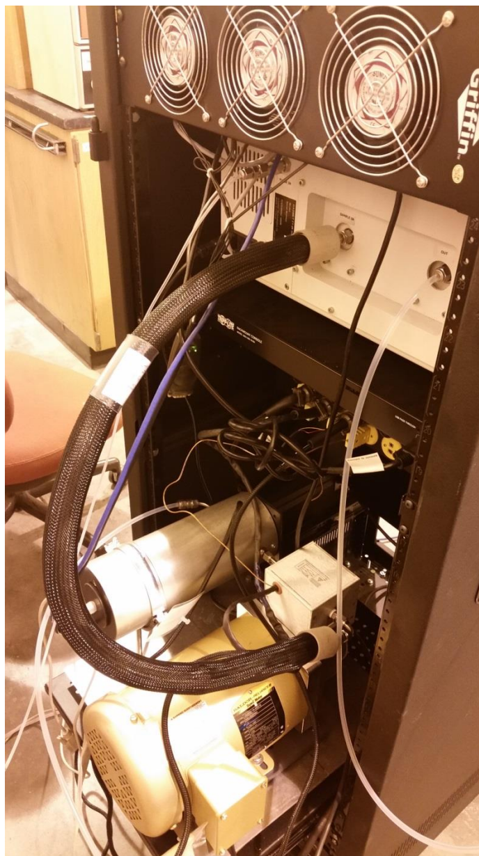
Figure A.11: Reverse side of CX-4000 analyzer cabinet. Sample inlet is next to the filter (Silver cylinder). From there, the sample is passed through the sample pump (Gold cylinder) and then the heated jumper line to the analyzer inlet. Power and thermocouple connections for heated components are visible as well.
