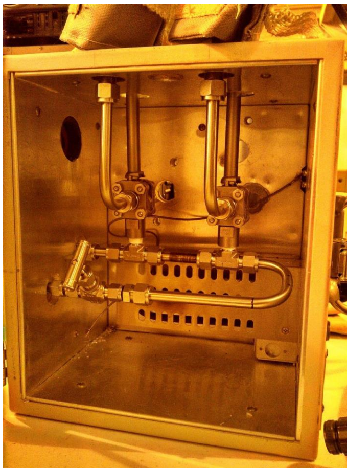
Figure 4.2: Heated sample switching box. Heated sample lines connect at the top of the box. Flow is selected through the 3-way valves and fed to the FTIR pump.
