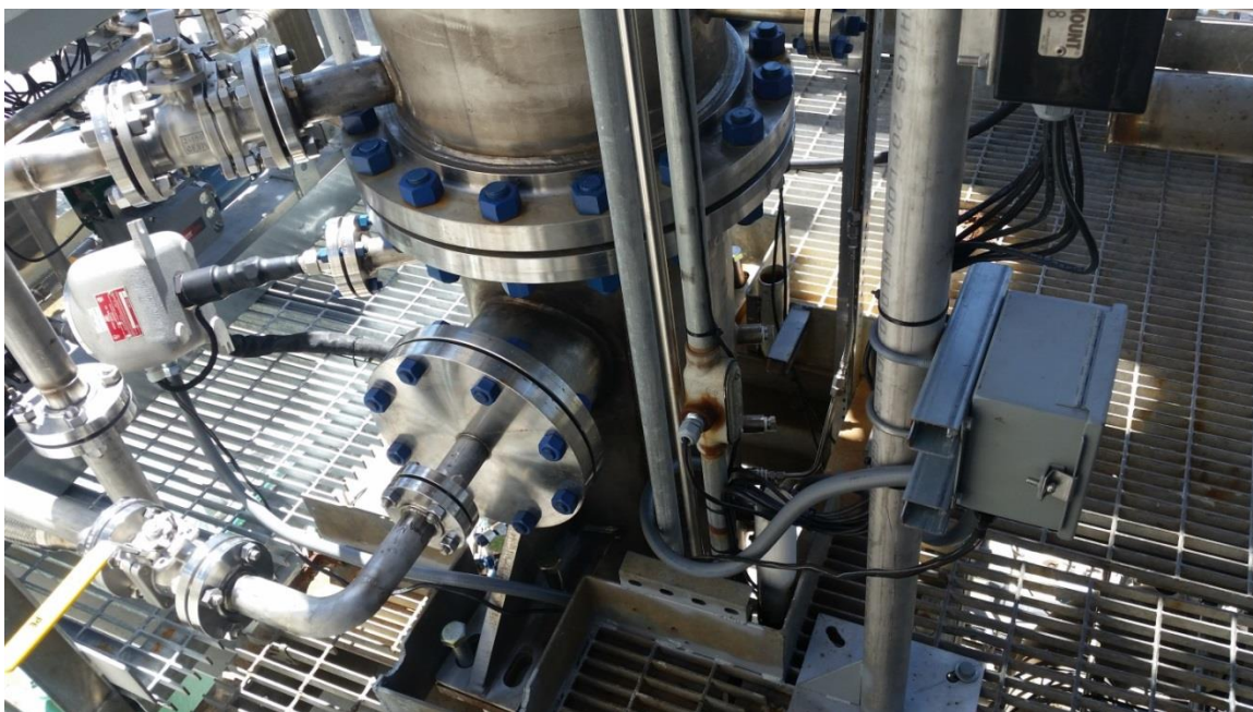
Figure 5.4: FTIR probe (to the left) for sample extraction between first and second stages of packing at UT-SRP pilot plant.
