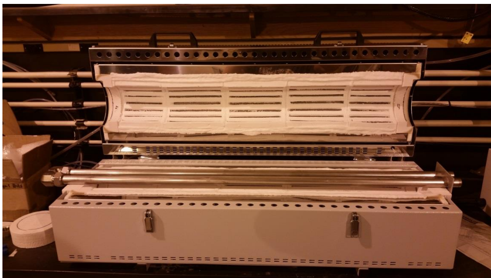
Figure 5.7: Heated tube furnace with catalyst bed for SO 3 generation
