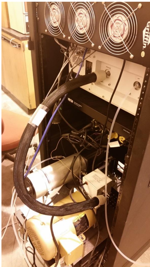
Figure C.2: FTIR in server rack from rear. The heated filter is the silver cylinder in the back. This connects to the heated pump head, the silver box. The heated sample line is the black hose from the pump head to the FTIR.
