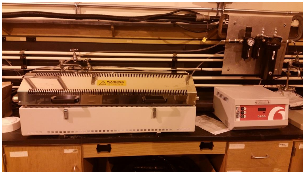
Figure 3.3: Carbolite HST 12/900 furnace with control unit (on right)
