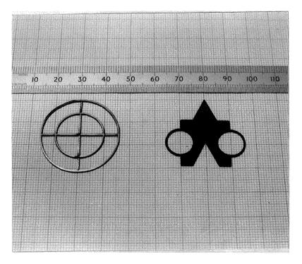
Figure 3. Laser cut parts in stainless steel
