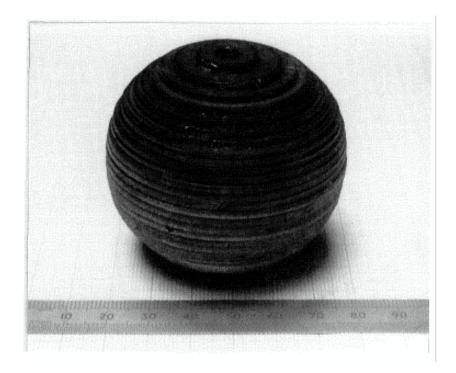
Figure 4. Sphere, produced in 2mm mild steel.
