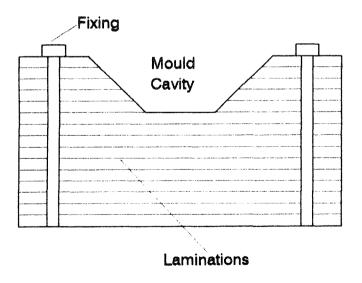
Figure 1. Typical arrangement for holding/fixing laminated tooling.
