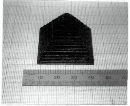
Figure 5. Square based hollow pyramid in 1mm thick stainless steel.
