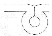
Figure 3: Toolpath generated by QuickSlice<sup>™</sup> for the interacting features of Figure 2 and the resulting part. Figure 3 describes the phenomenon in a toolpath generated by QuickSlice<sup>TM</sup>. An expected hole is not completed in the fin structure. Unless thickness of the road is larger than designed, the gap may not fill. Moreover, a seam will be present at the juncture of the two sharply turning roads.
