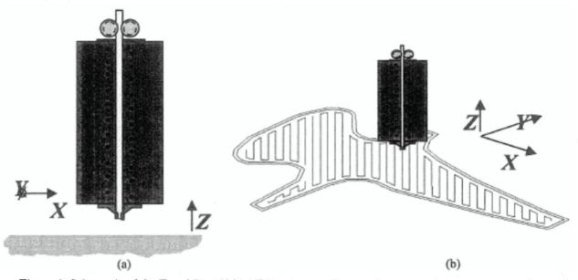
Figure 1: Schematic of the Fused Deposition (FD) process. To the left (a) is a close up of a straightened liquefier, showing the material being deposited on a flat platen to form the part. At right (b), the tool is shown traversing a path that describes the cross section of the part.
