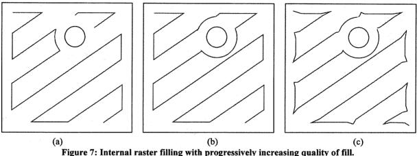
Figure 7: Internal raster filling with progressively increasing quality of fill.
