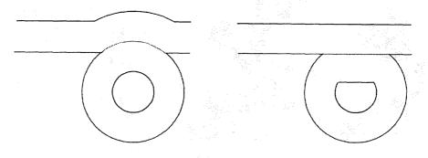
Figure 4: Two options of the new toolpath giving the designer control over feature retention. On the left the circularity of the hole is preserved, while on the right the fin surface is preserved.
