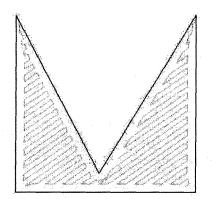
Figure 6: Raster toolpath for a doublewedge with no external perimeter.
