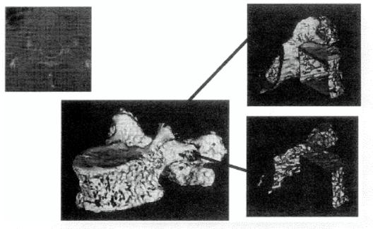
**Figure 4.** Inset: Original MRI image; composite model representing outside shell of dense bone and inside spongy bone. Composite model is constructed to allow filling of different materials to create non-homogeneous final product.
