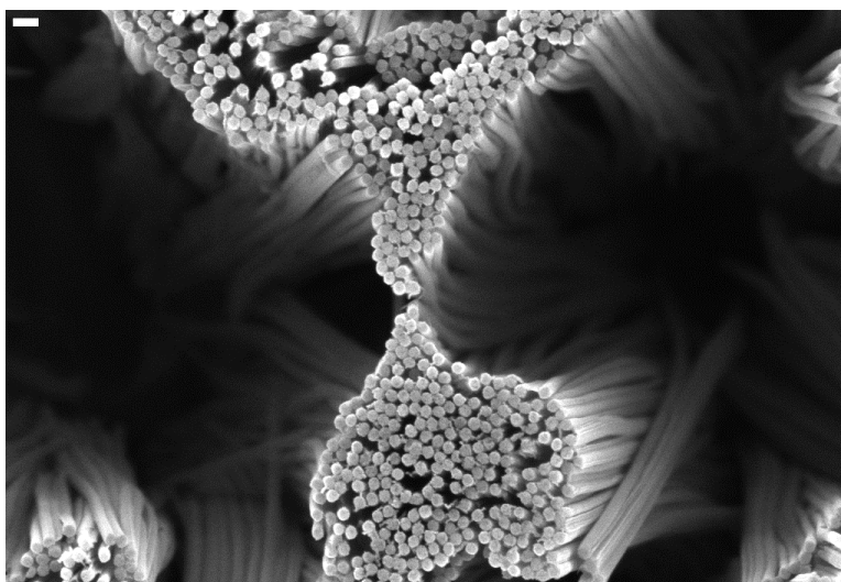
Figure 4-22: Top down view of collapsed circular pillars. Scale bar is 200 nm.
