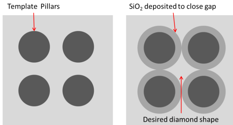
Figure 4-11: Diamond shape created by ALD deposition on template with circular nanoscale pillars.
