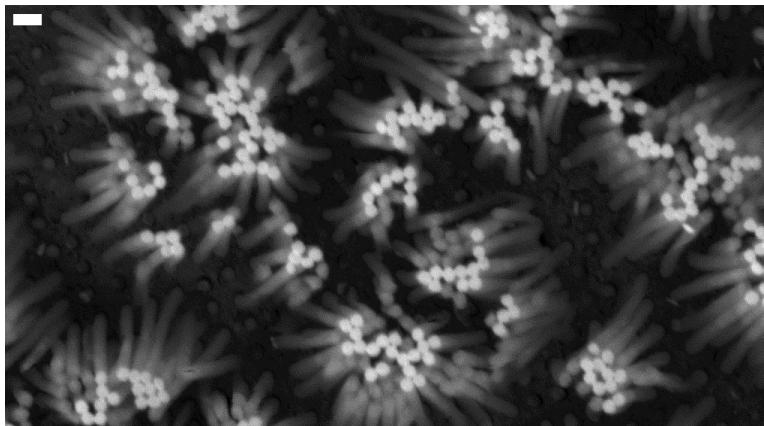
Figure 4-10: Nanowires fabricated using gold mesh fabricated using bi-layer lift-off process. Scale bar is 200 nm.
