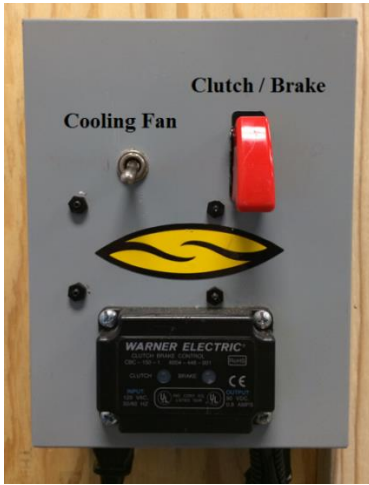
Figure 3.5: Power unit for the cooling fan and clutch brake.
