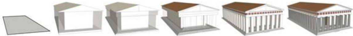
Figure 9: Generation of building geometries with CGA shape grammar, Source: (Esri R&D Center, 2017)
