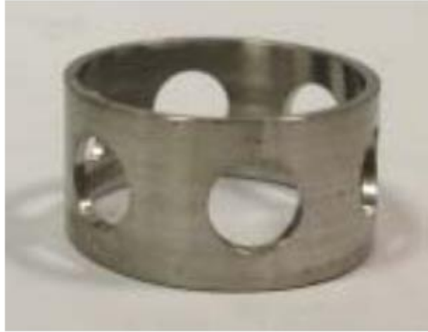
Figure 2- 4 General purpose disintegrating head (Kumar et al. 2013)
