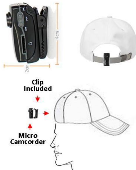
Figure 3. Method for Mounting Micro-Camcorder
