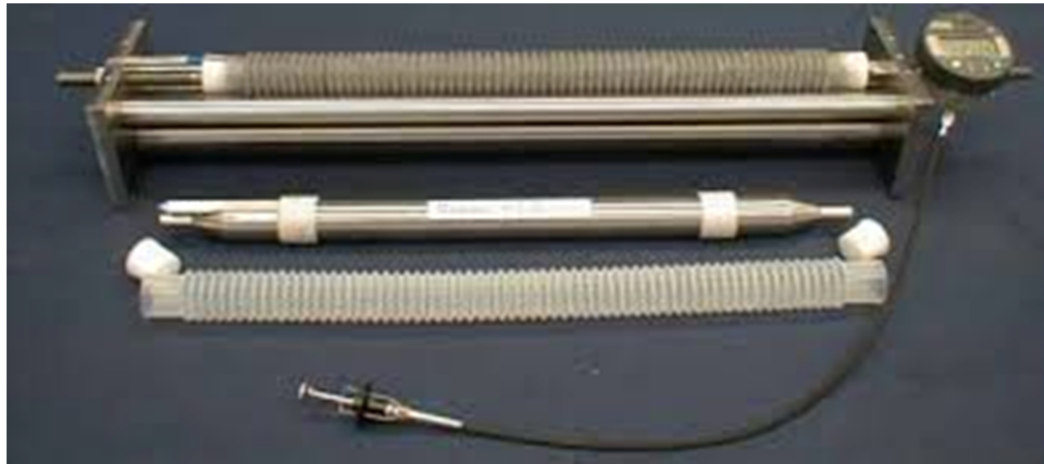
Figure 11: Corrugated polyethylene autogenous test setup (Germann Instruments)
