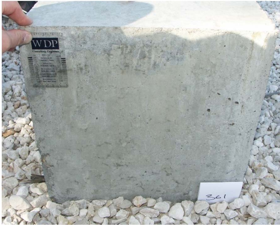
Figure 92: Example Crack Rating = 2
