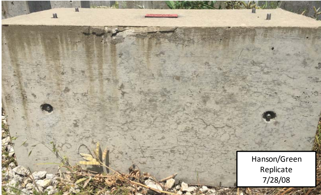
Figure 3: Precast plant straight cement exposure block replicate cast according to ASTM C1293 0.45 w/cm
