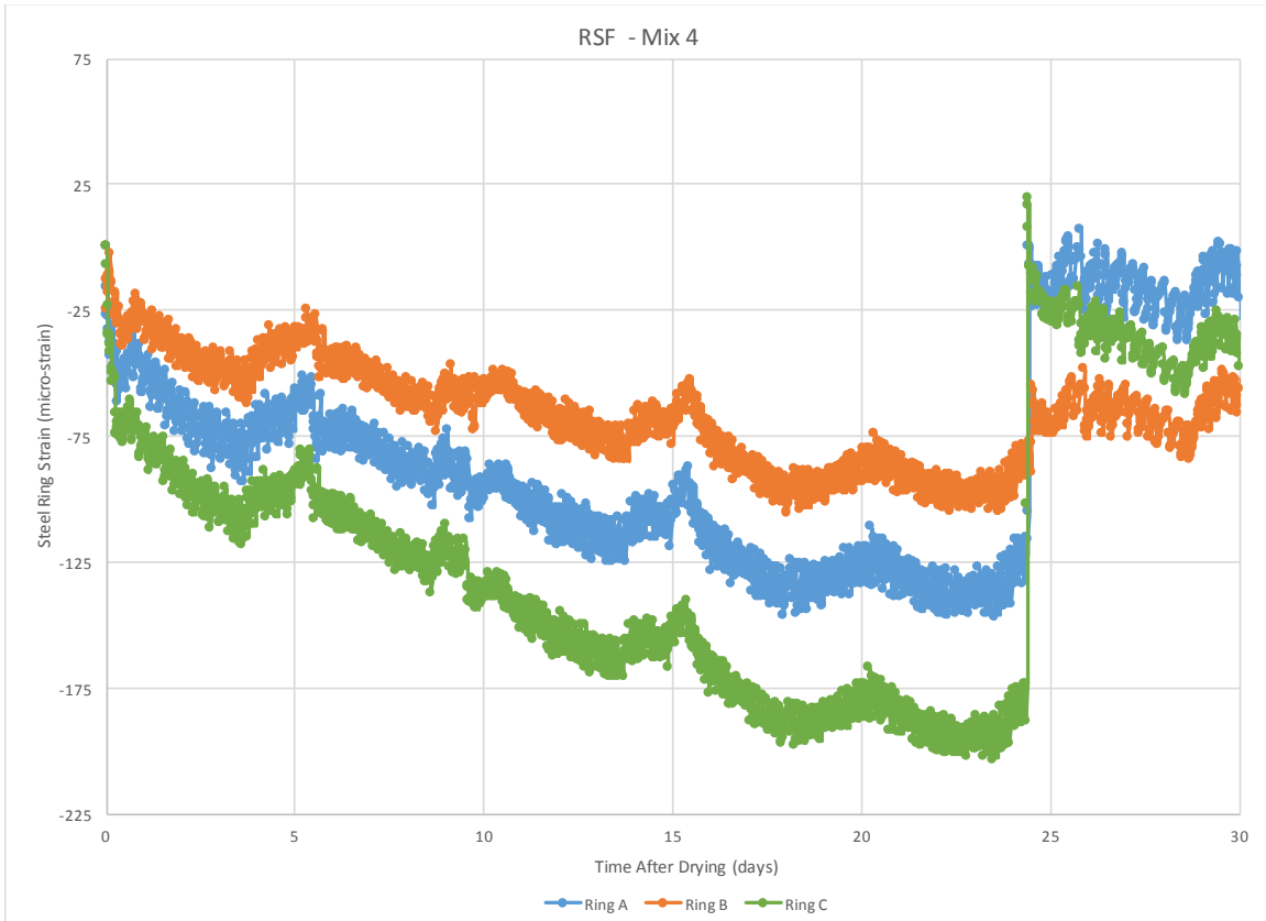
Figure 155: Net strain vs time (days) for rings A, B and C for Mixture 4
