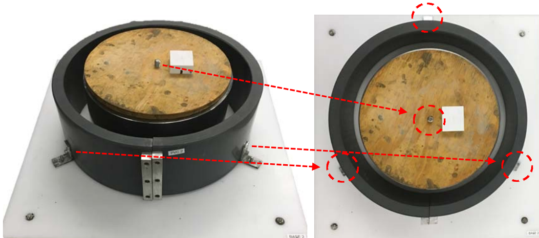
Figure 40: Locking locations for securing the inner and outer rings to the restrained shrinkage ring bases denoted in red
