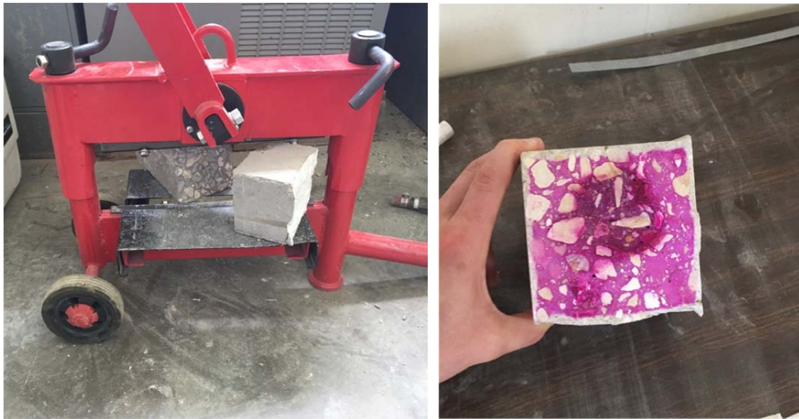
Figure 18: (Left) Device used to cut concrete carbonation specimens. (Right) Phenolphthalein sprayed specimen and depth measurement front
