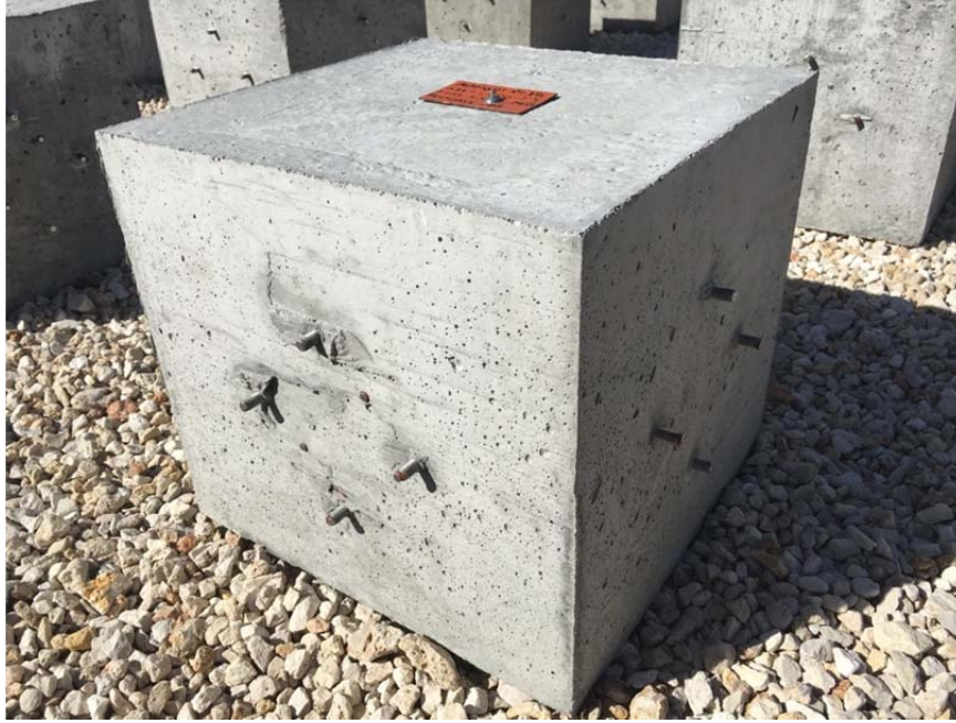
Figure 110: Exposure Block with Expansion/Shrinkage Measurement Locations
