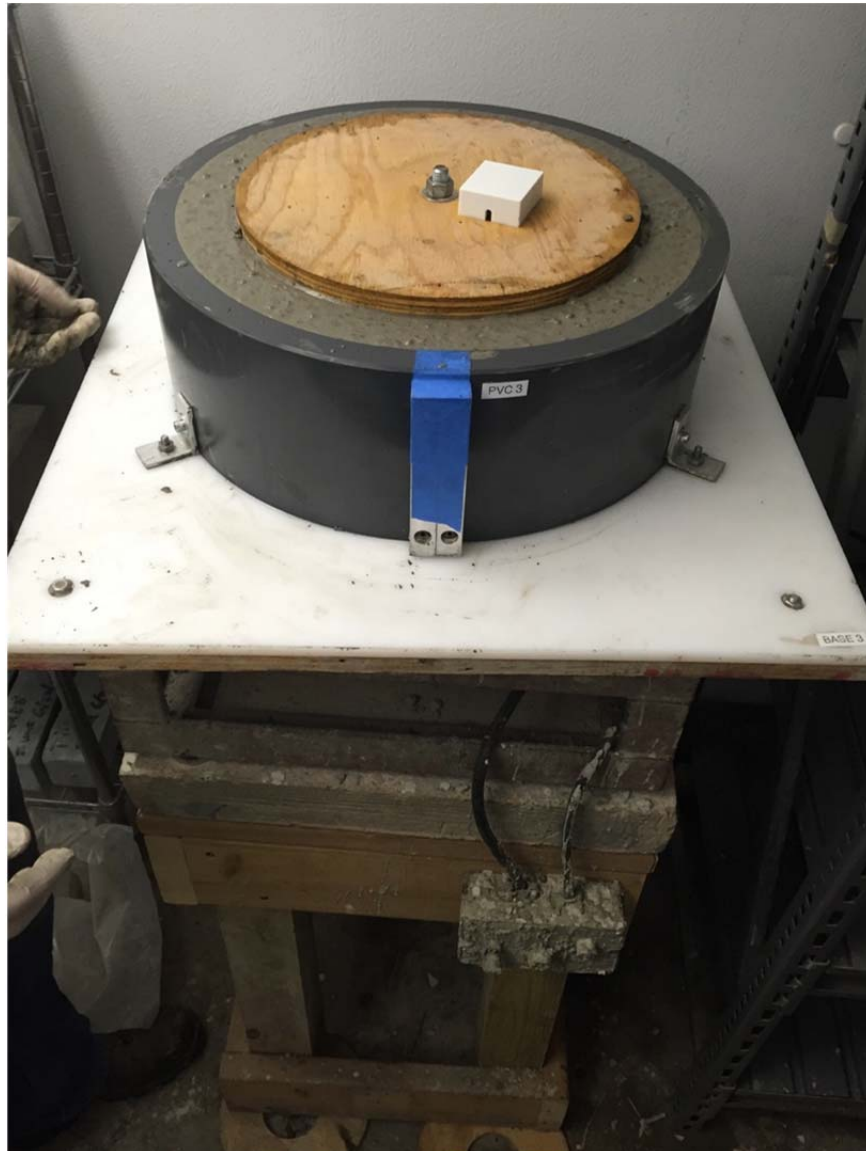
Figure 45: Casting restrained shrinkage ring on vibrating table
