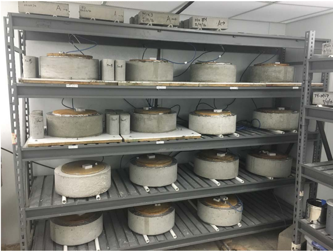
Figure 46: Restrained shrinkage rings (4 mixtures), Monitored in the testing room
