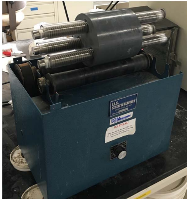
Figure 74: Automated turning apparatus for reducing bleeding on corrugated tube sample
