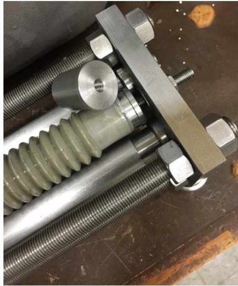
Figure 75: Stainless steel end caps used for the version 1 setup to facilitate shrinkage solely from measurement end
