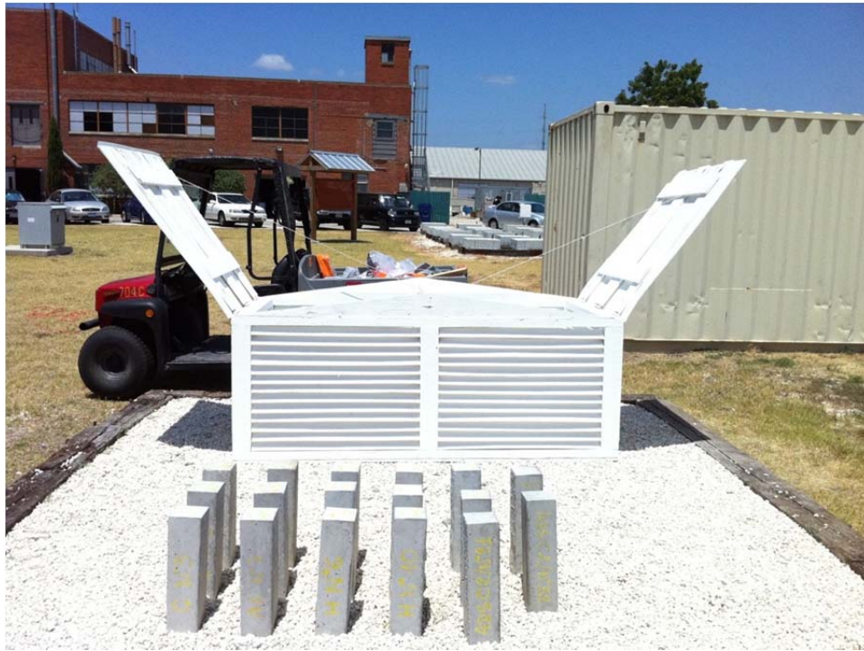
Figure 109: Carbonation exposure site at UT Austin with shelter (Stevenson Screen)
