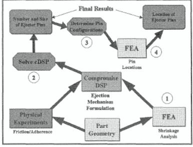
Figure 2 Process Flowchart
