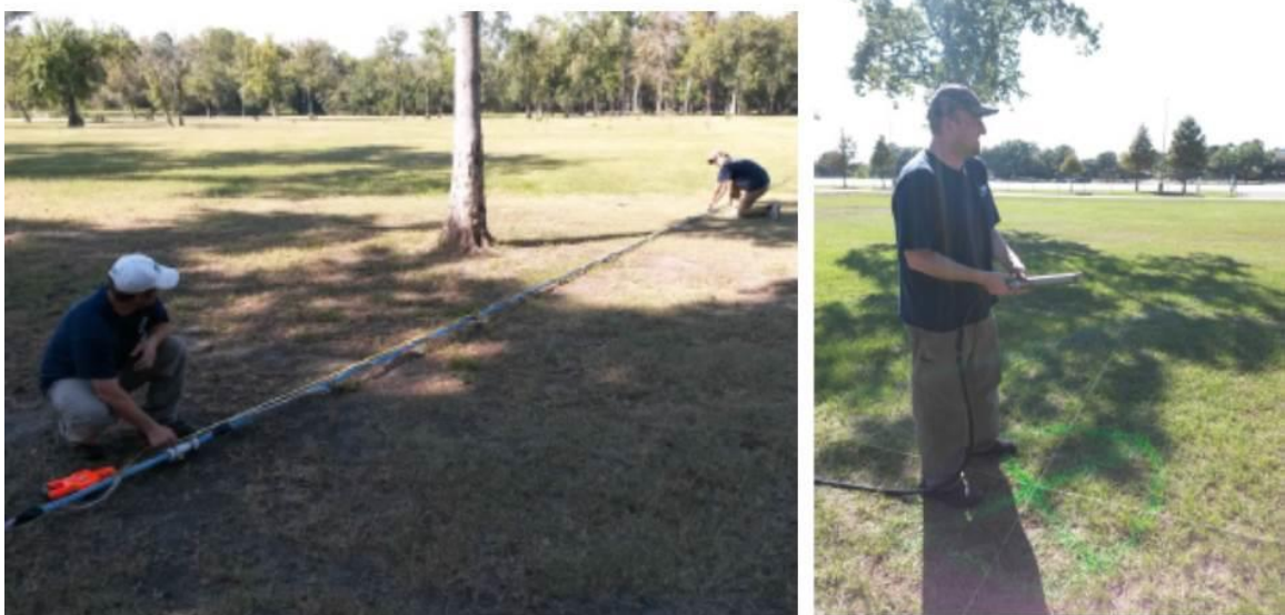
Figure 2.9 – Left: measuring streamer offset with 1500lbs of tension. Right: tail compass calibration at magnetically quiet test site. Images from UT P-Cable Nav GoM 2013 report.
