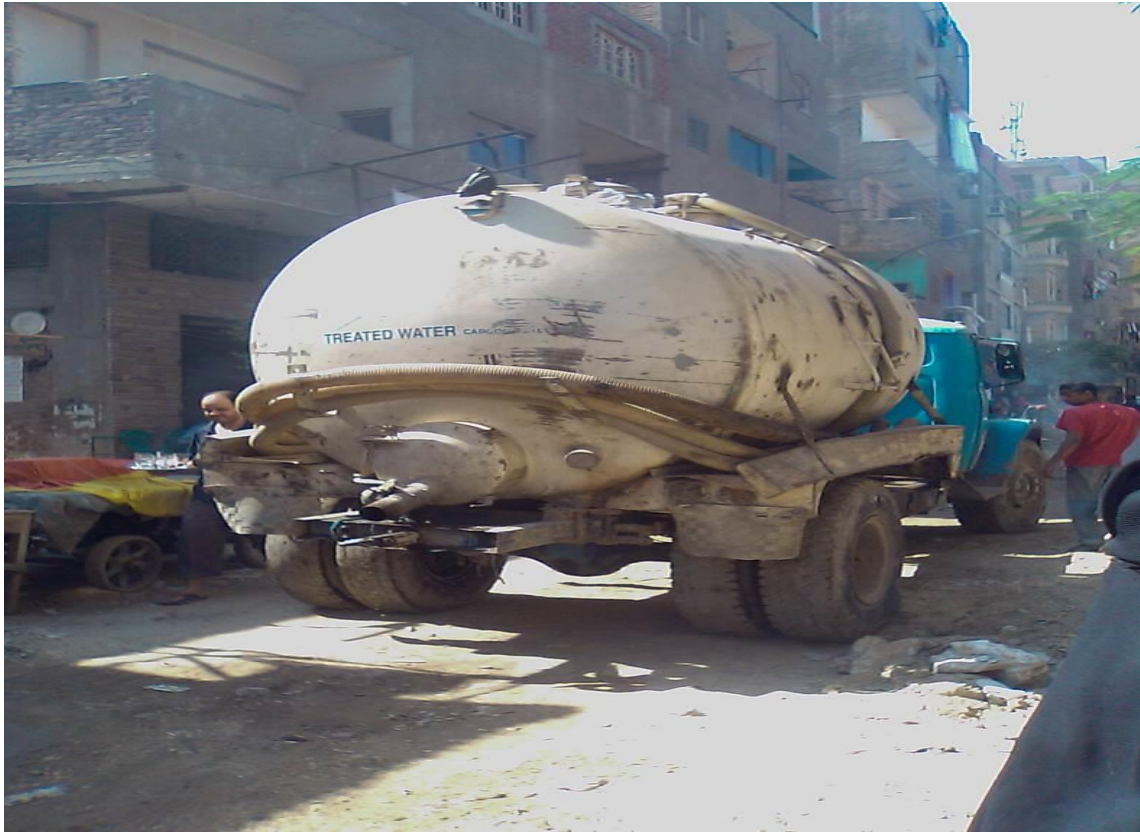
Figure 13: Septic tank removal truck in Ezbet Khairallah. Image by author, 2010.
