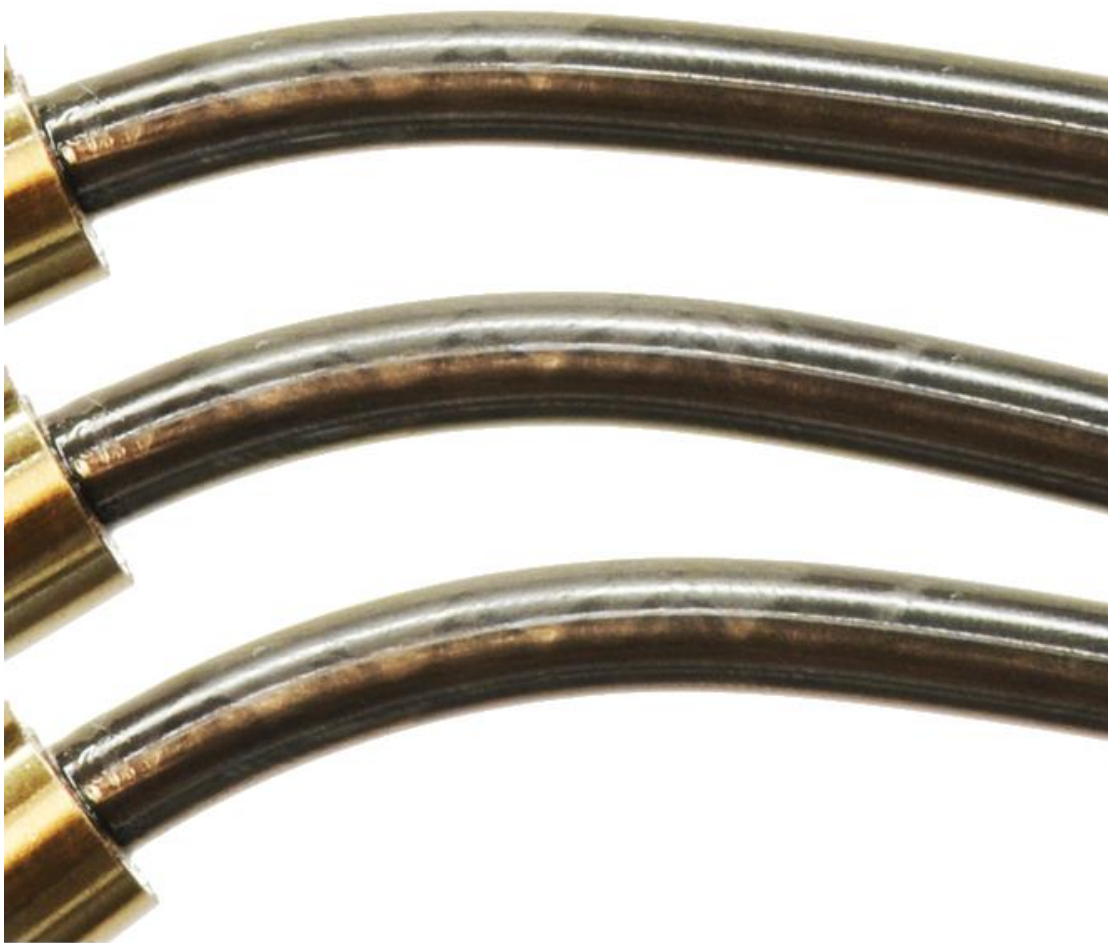
Fig. 3.5 Expanded view showing the evolution of diamond deformation patterns on the tensile side of the tube in Figs. 3.3 and 3.4.
