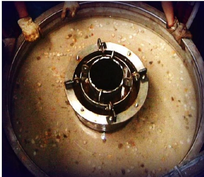
Figure 4.11: Laboratory formation used to simulate invasion of 200-kppm [NaCl] brine into a fresh water saturated 34-p.u. sandstone. The metallic cylinders in the center of the sandstone block are 1-mm thick steel liners used to physically separate virgin and invasion zones. These liners affect measured multi-detector time decays.
