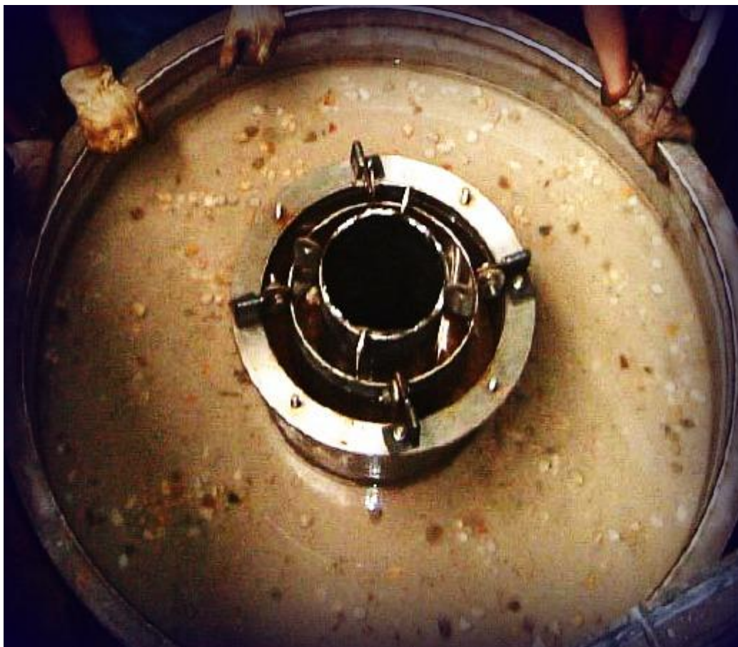
Figure 3.5: Experimental facility used to emulate piston-like invasion. The concentric steel liners are used to physically separate virgin- and invasion-zone fluids.
