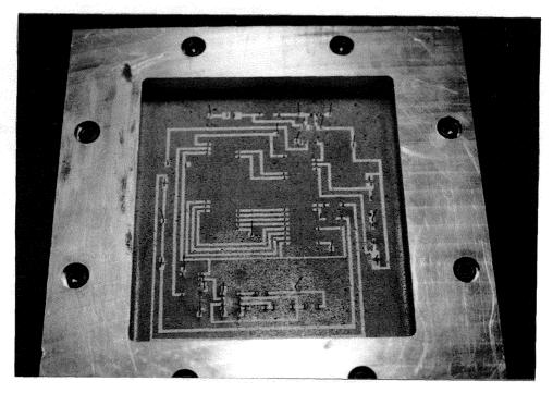
FIGURE 4. Sprayed Interconnections: Layer 1
