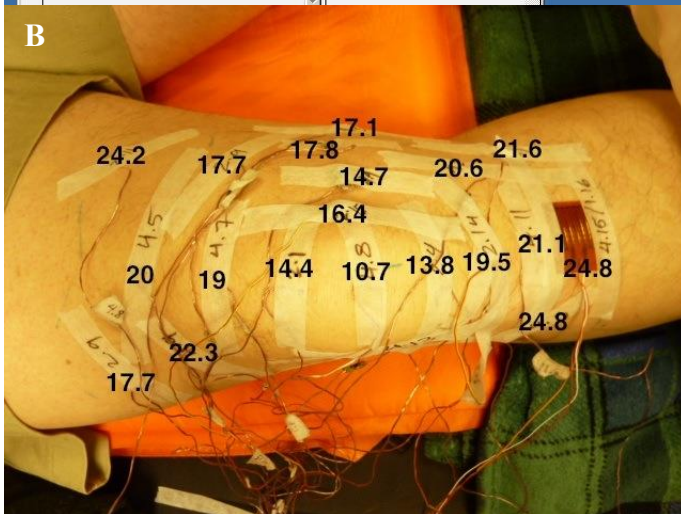
Figure D. 2. The skin temperature in the treatment region at the end of cooling from the frontal aspect using IR imaging (a) and thermocouple readings (b). The thermocouple measurements show minimum temperature measured at each location.
