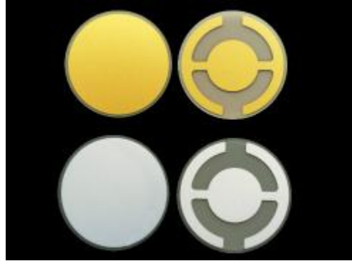
Figure 3.7: A quartz crystal microbalance is used to calibrate the metal fluxes prior to deposition. Taken from [11]
