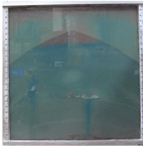
Figure 4.30: The aqueous reservoir connected to the bottom was brought back to the original position (the same level as top of the domain) while the oil collecting reservoir was raised 5 inches higher to drive backflow of oil along connected pathways into the apparatus and into the accumulation remaining in the coarse beads beneath the fine beads. In the absence of such a pathway, no change in the oil accumulation is expected. No back flow occurred, confirming that the oil displacement from the coarse beads into the fine beads is controlled by capillary pressure, not by viscous fluid gradients.
