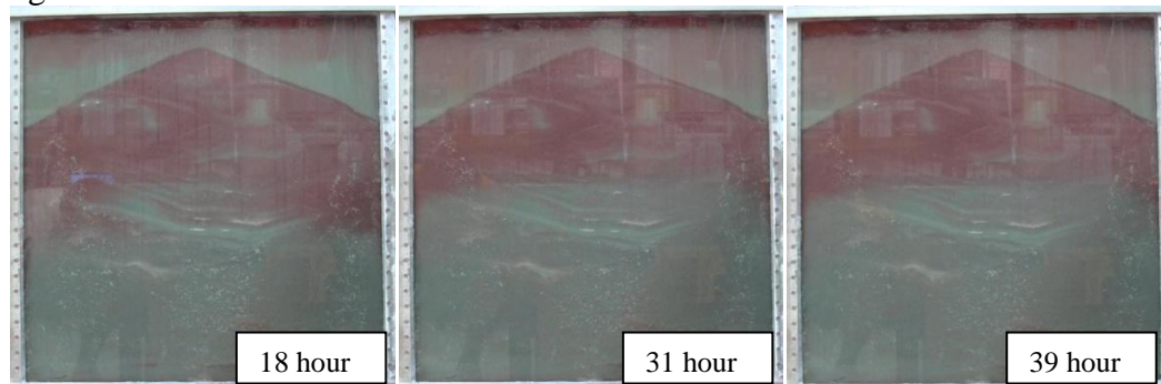
Figure 4.24: Late time equilibrium state (insets give elapsed time since start of buoyancy-driven displacement in closed system) of the open system of experiment 8. Constant hydraulic potential equal to hydrostatic was applied at top and bottom ports at the 8 th hour elapsed time.
