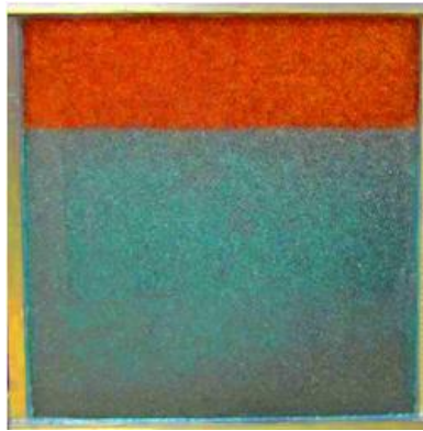
Figure 3.10: Initial condition of the closed-state experiment. After packing granular medium of hydrophilic beads in the apparatus, aqueous phase (blue) (the brine/glycerol mixture) was slowly injected from the bottom to fill entire medium, followed by slow injection of light mineral oil/decane mixture (red) from the top to displace aqueous phase through the bottom. To initiate the buoyancy driven displacement, the gravity-stable configuration shown in this photograph is reversed by pivoting the apparatus 180 degrees in the frame (a rotation around a horizontal axis through the middle of the domain in the photograph), thus the denser aqueous phase is placed above the less dense hydrocarbon phase.
