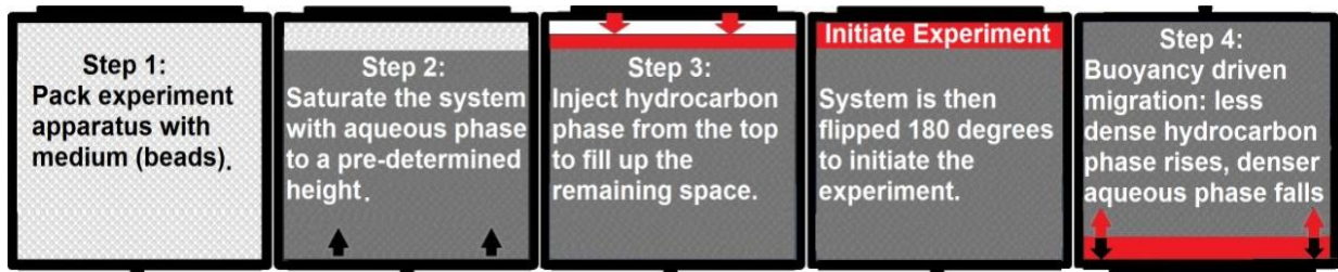
Figure 3.9: A graphical representation of the closed-boundary experimental design. The design calls for emplacing the nonwetting phase in a gravity-stable manner (filling from the top), closing valves, then flipping the apparatus to start the buoyancy-driven displacement.
