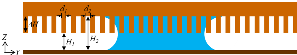
Figure 4.20: Schematic showing template with line and space patterns with width d_1 and d_2 respectively. The minimum and maximum gap between the template and the substrate at any time is H_1 and H_2 respectively.
