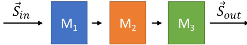
Figure 4.3: The diagram above depicts polarized light propagating through three distinct media, each described by their own Mueller matrix. The output polarization state of light can be calculated if the input polarization state and Mueller matrices for each element are known ( EQ 4.5 ):
