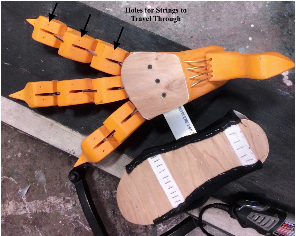
Illustration 21: Holes for Strings to Travel Through
