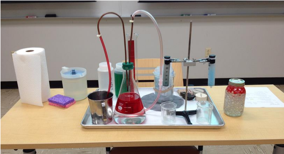
Figure 17: Injection and production well demonstration (Dees, 2014).
