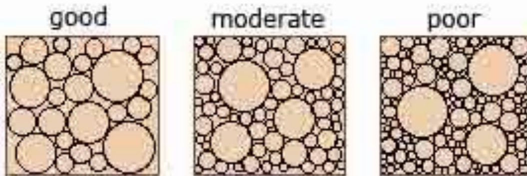
Figure 8: Example sorting arrangements of sand grains in sandstone (The Open University 2014).
