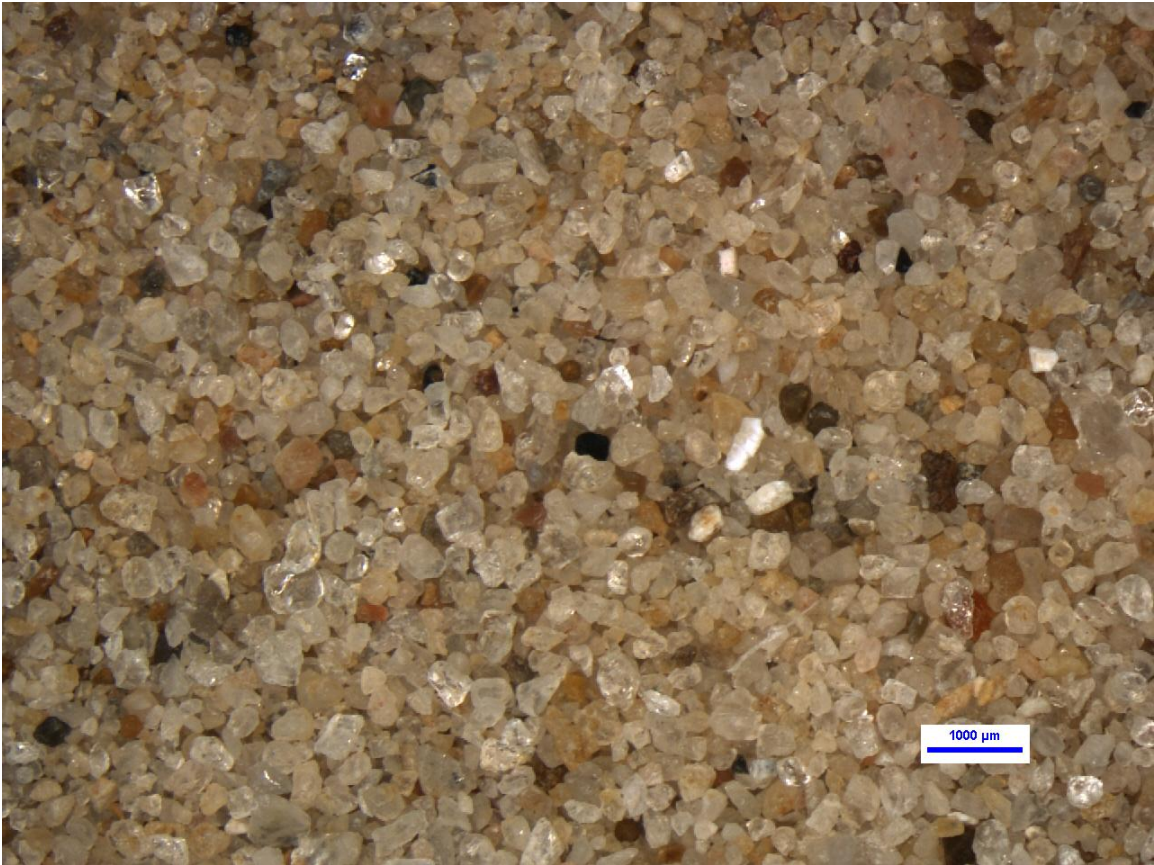
Figure 35: Sand grains from the mortar sample viewed at 10x.
