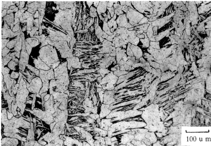
Figure 6 - Large equiaxed Ferrite and Pearlite structure
