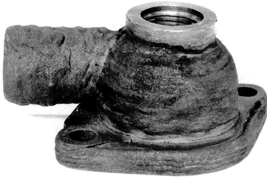
Figure 3 - Welded Thermostat Housing
