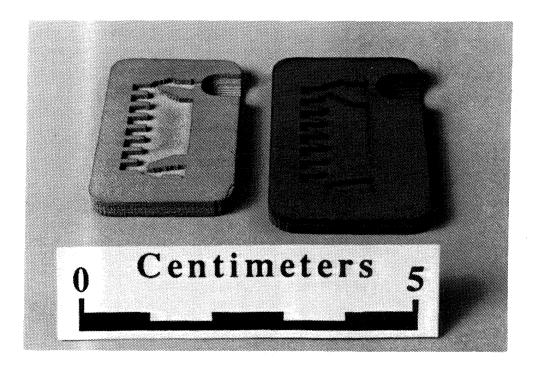
Figure 5. A 3D Printed Part Sintered to 78% Density (left) and a Green Part (right).
