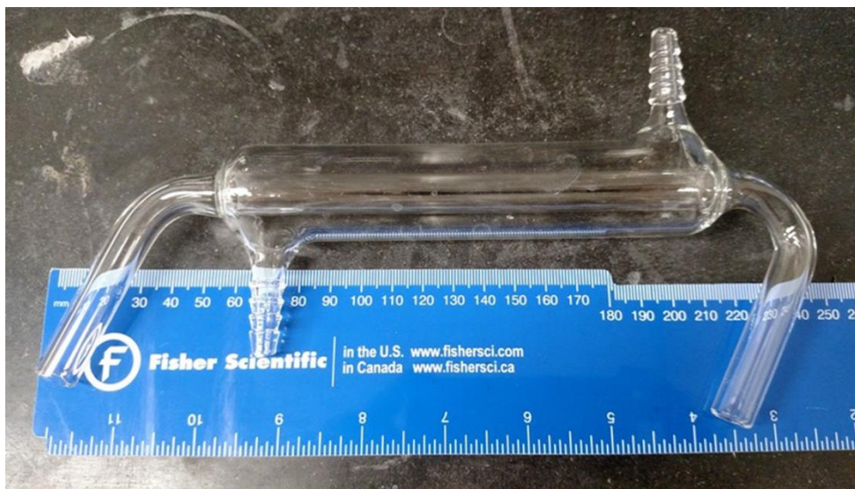
Figure A.4: Photograph of angled distillation head (shown with jacketed condenser).
