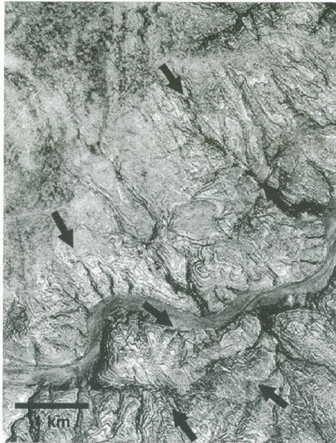
Figure 4.2(a): The sharp, linear features indicated by arrows are fracture zones. Note the many similar features parallel to those indicated. Also note the fracture controlled stream courses.
