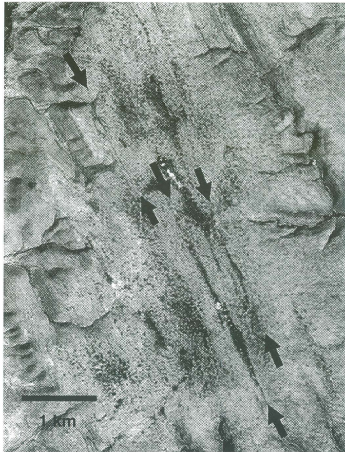
Figure 4.2(c): Linear vegetation trends. Fracture zones are typically more weathered than surrounding rock, allowing relatively lush vegetation.
