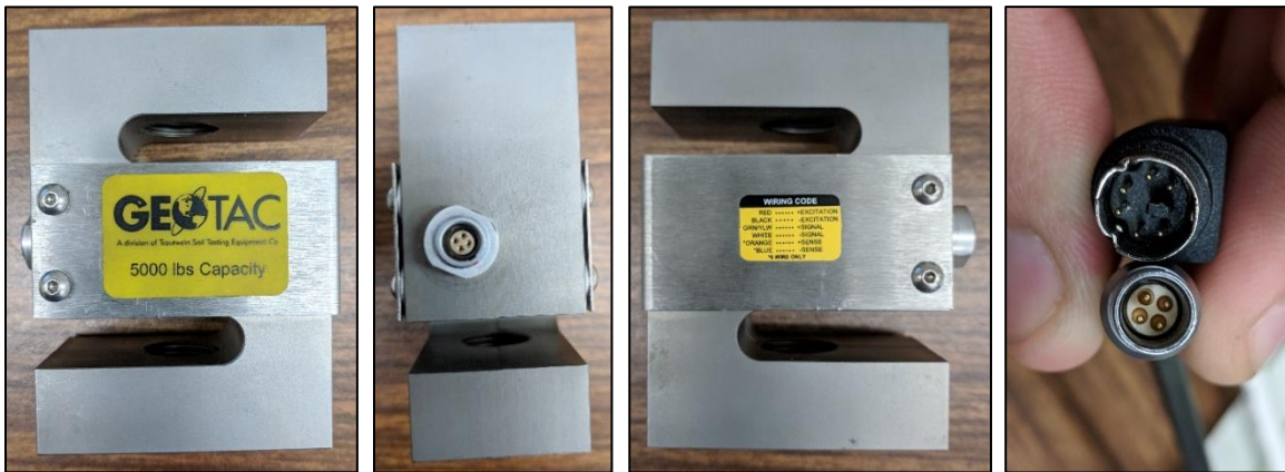
Figure 81. Front, side, and rear view of Geotac 5k load cell and 4-pin male & 6-pin mini DIN male cable ends provided by the manufacturer
