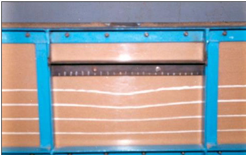
Figure 12. Post-test deformation pattern of subgrade soil underlying a geocell mattress, (Dash 2012)
