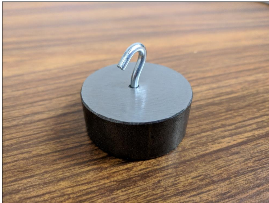
Figure 42. Steel hanging weight with hook to compensate for nominal draw wire tension
