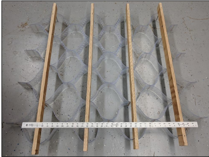
Figure 24. Transparent PVC geocell test section of GC 1 with 150-mm depth (PVC GC 1-150)
