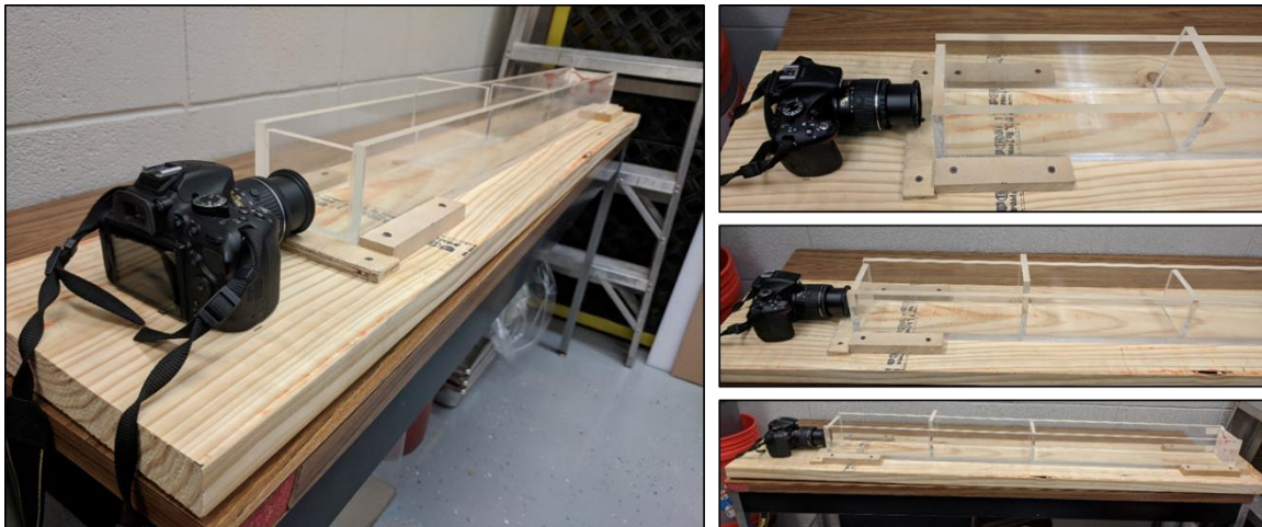
Figure 58. Full-depth transparent soil apparatus
