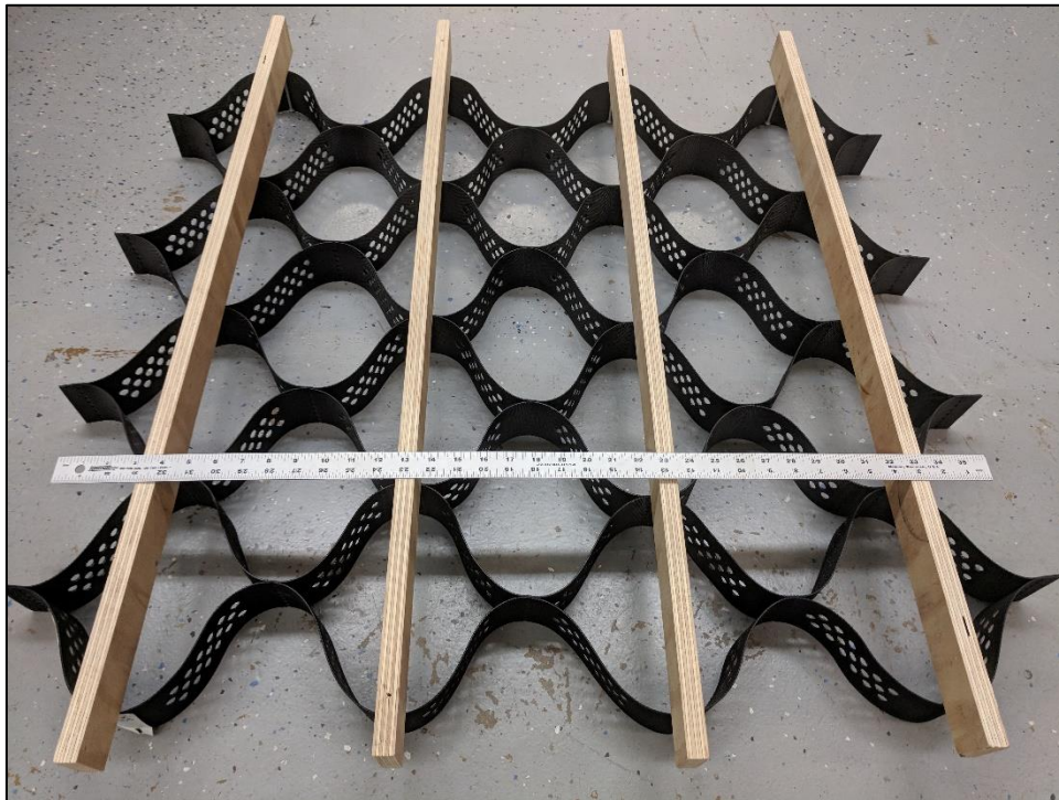
Figure 23. Textured HDPE test section of GC 1 with 150-mm depth, (HDPE t GC 1-150)
