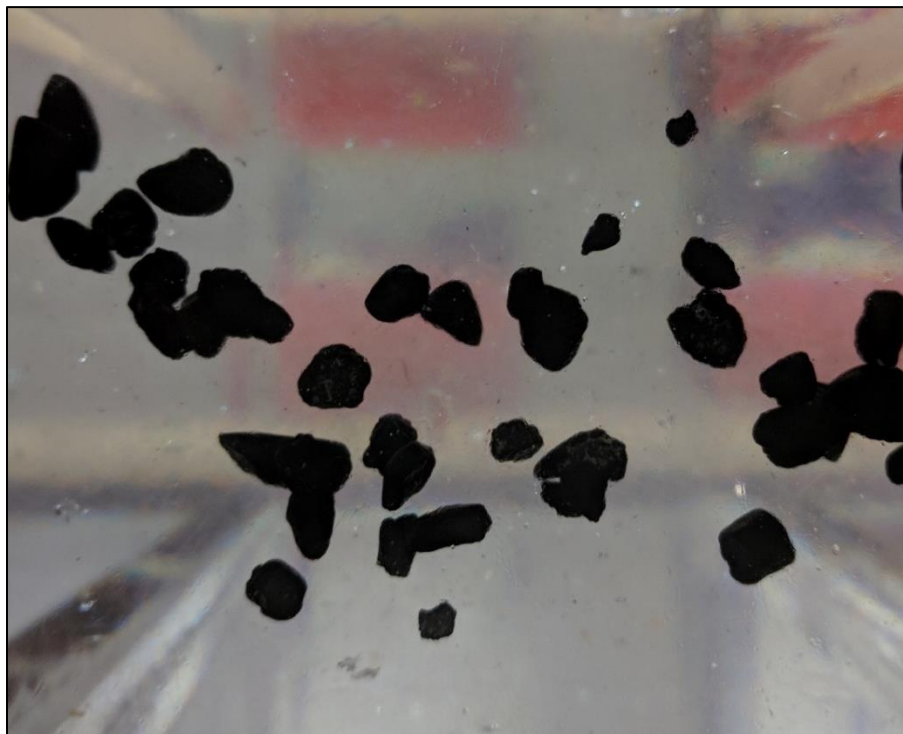
Figure 31. Opaque soil particles suspended in transparent soil
