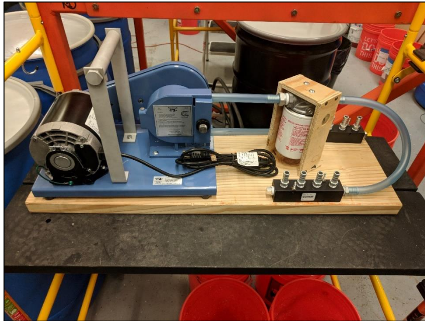
Figure 45. Pump, filter, and manifold assembly as part of the oil circulation system
