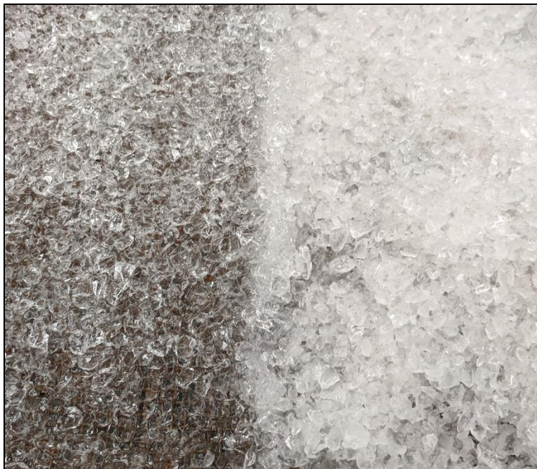
Figure 29. Processed (left) and raw (right) crushed fused quartz
