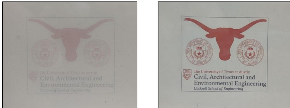
Figure 50. Comparison of oil clarity before and after oil filtration of micro-contaminants
