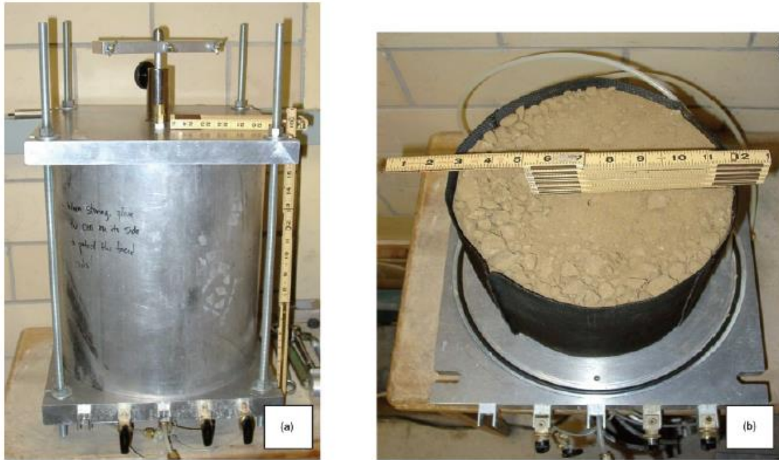
Figure 20. Large-scale resilient modulus testing apparatus: (a) side view of assembled cell; (b) top view of unassembled cell with specimen confined in geocell
