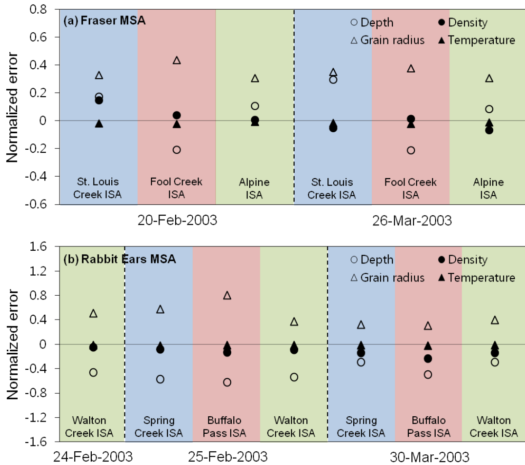
Figure 2.8. Normalized errors ( = (\text{simulation} - \text{observation}) / \text{observation} ) of snow depth, density, grain radius, and temperature for each ISA within the Fraser and Rabbit Ears MSAs. Since both observations and simulations showed dry snowpack conditions, normalized error of wetness is not shown.
