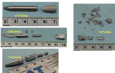
Figure 3. Projectiles broke into more pieces at higher velocities.
