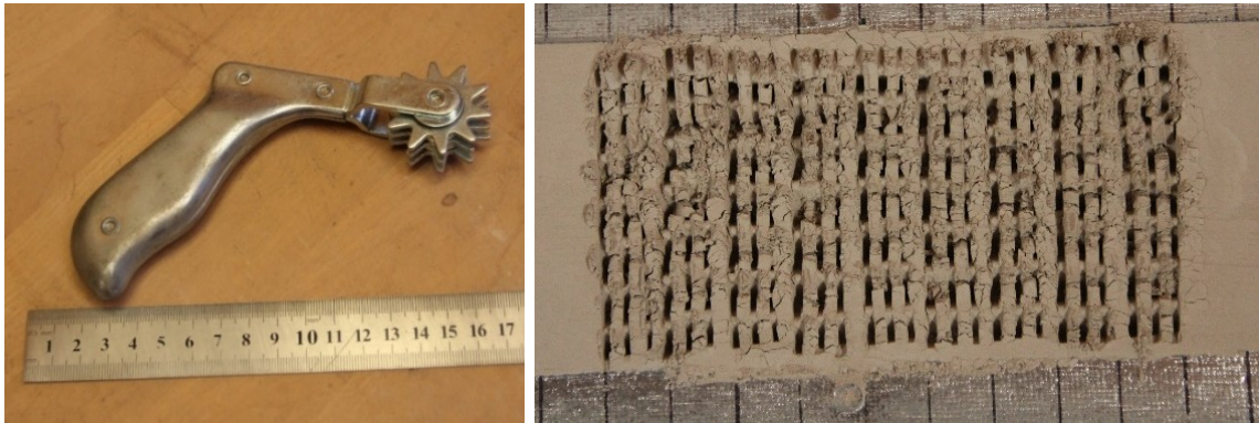
Figure 4.4. Dressing tool used for roughening the soil surface (left) and a sample picture of the rough surface created for the clay soil (right).
