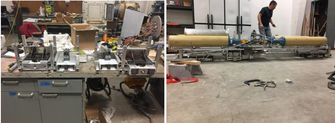
Figure 3.7 a) The brake frames (left) are shown having been installed into the full pod (right)
