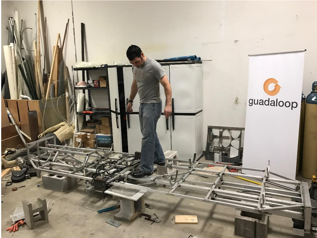
Figure 3.3: Texas Guadaloop’s welder standing on the frame, showing its robustness and lack of deflection at its most vulnerable point
