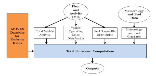
Figure 4.1: The MOVES approach to mobile source emissions estimation
