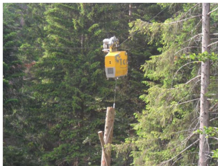
Figure 2.5 TECNO Intelligent Crane Carriage Retrieving Felled Timber
