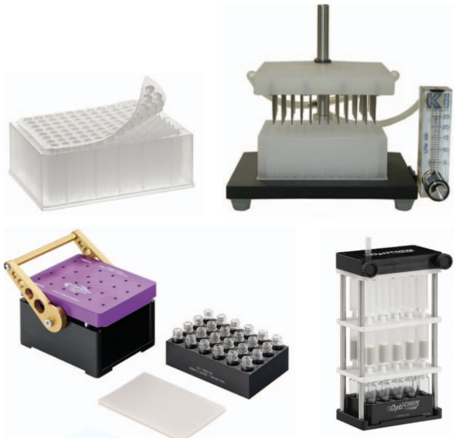
Figure 1.2: Tools for parallel synthesis. Clockwise from the top left: 96-well plate with sealing caps, Evaporator/manifold system in multi-well block, parallel synthesis reaction block, parallel purification tower.
