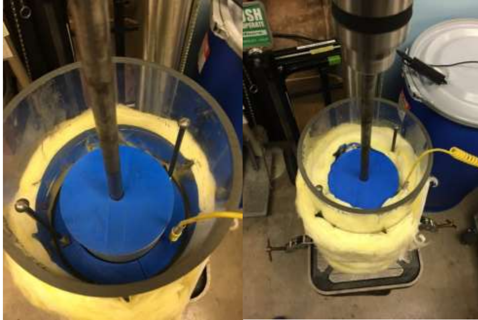
Figure 20. Halbach Heating Test Set-Up.
