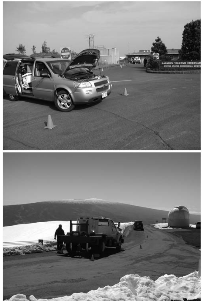
Figure 3. (a) SASW survey in the parking lot at the Hawaiian Volcano Observatory (HVO). Recording and analysis van is in the foreground and Thumper in the far background. (b) Thumper at the top of Mauna Kea. Mauna Loa is in the background.
