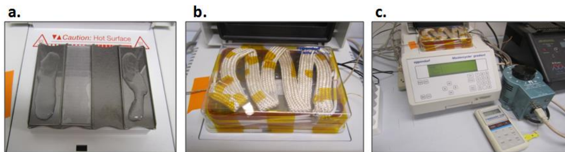
Figure 7.10. Images of a. the poorly-sealed microwell chip loaded into PCR b. the modified PCR lid and c. the custom temperature feedback system.
