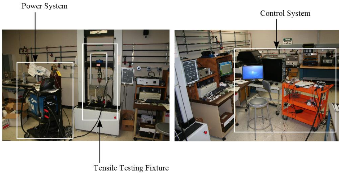
Figure 2.6: Schematic representation of the direct electrical resistance heating system (top) and photographs of the direct electrical resistance heating system (bottom).
