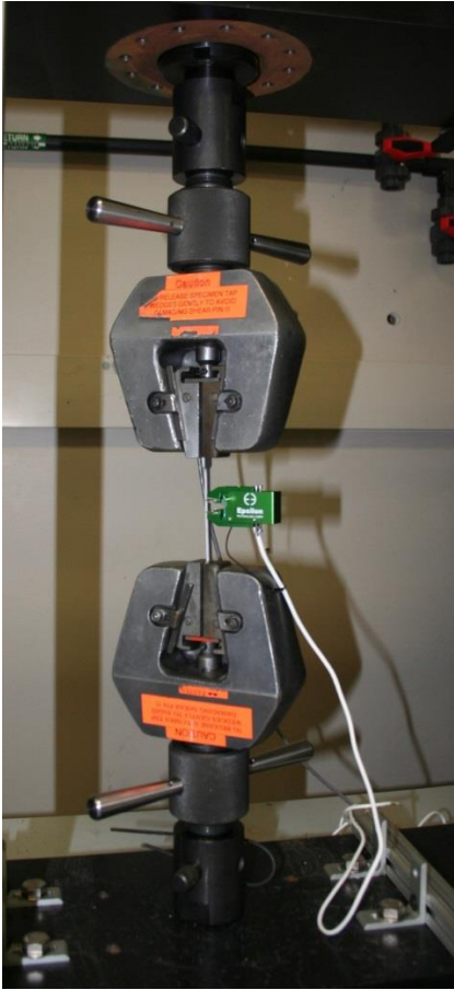
Figure A.22: Photograph of the room-temperature tensile testing setup.
