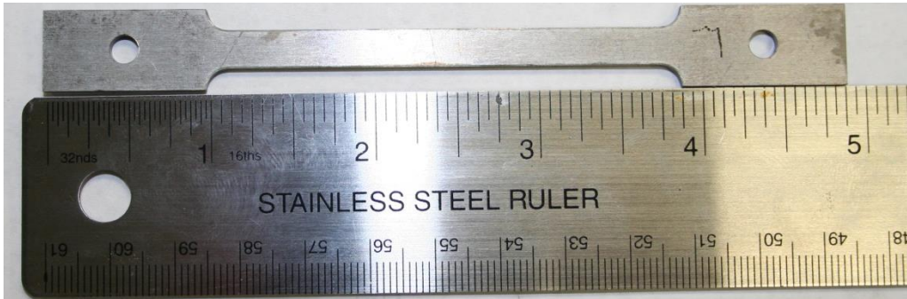
Figure A.21: Photograph of the tensile coupon used for room-temperature tensile tests.
