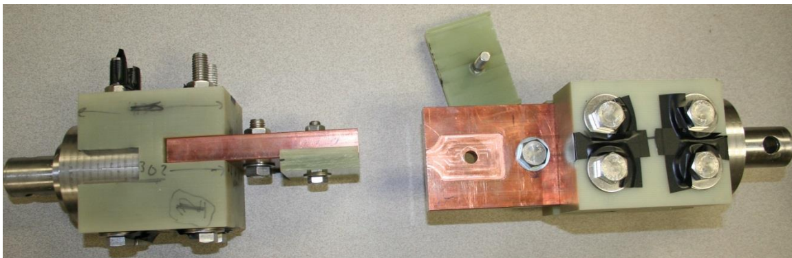
Figure A.27: Direct resistance heating tensile grips.
