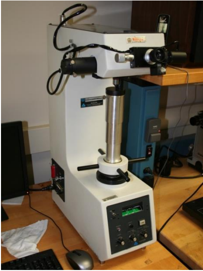
Figure A.4: Buehler Macro Hardness Tester, Model 1900-2005 used for hardness testing.
