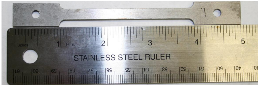
Figure A.23: Photograph of the tensile coupon used for solution-temperature tensile tests.
