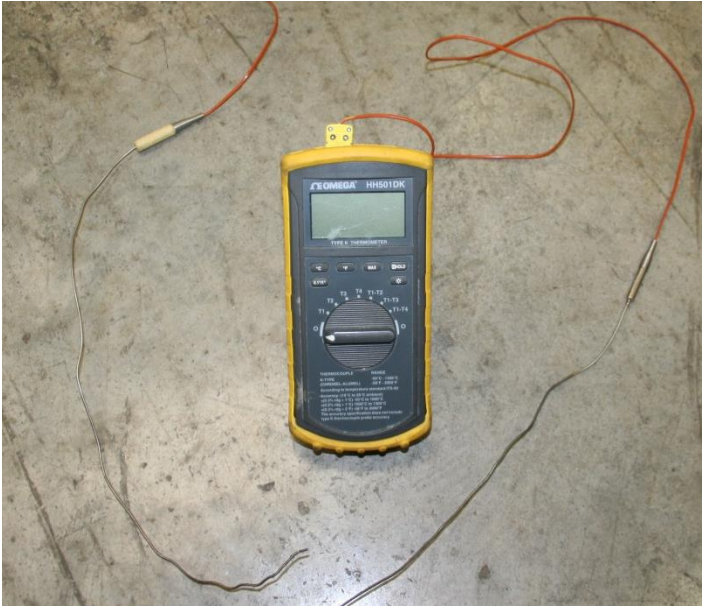
Figure A.3: Omega HH501DK hand-held thermocouple readout and metal sheathed type-K thermocouples.
