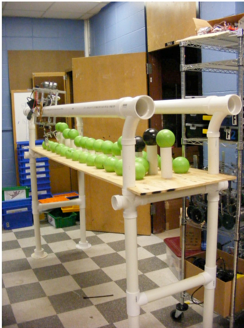
Figure 3.1: Rail robot perched on rail and shelf system.
