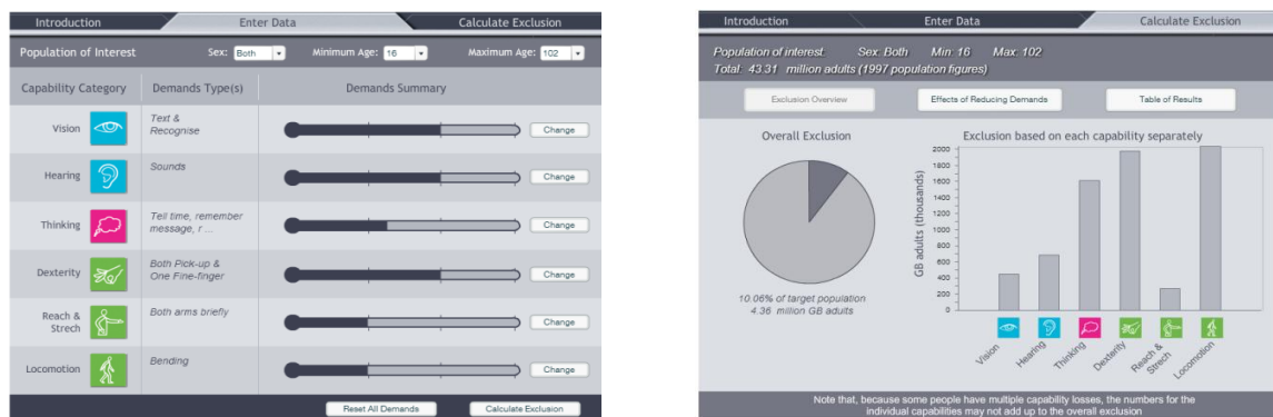
Figure 4: Screenshots of Exclusion Calculator, from Inclusive Design Toolkit. On left is the Enter Data page to select the various set of capabilities related to any product. On right is the result of the Exclusion which shows the number of people based on various capabilities such as vision, hearing, thinking, dexterity, reach & stretch and locomotion, http://www.inclusivedesigntoolkit.com/betterdesign2/exclusioncalc/exclusioncalc.html , Accessed on May 4, 2015.(© Copyright University of Cambridge 2013)
