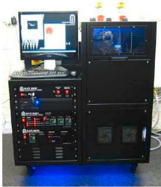
Figure 4.10: Black magic system by Aixtron for growing graphene by chemical vapor deposition.
