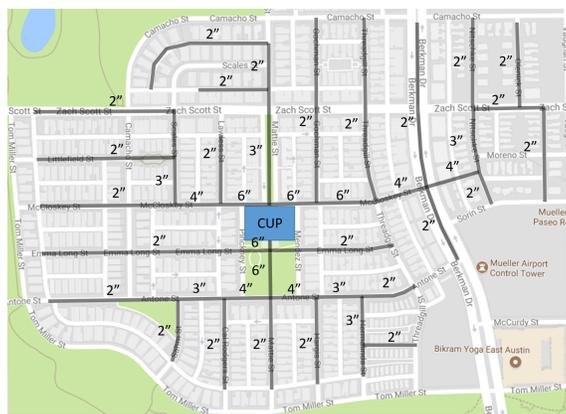
Figure 6.9: A rudimentary design for the neighborhood chilled water distribution system using design guidelines from [165] helps estimate the capital cost of the piping network at \$2.9 Million.
