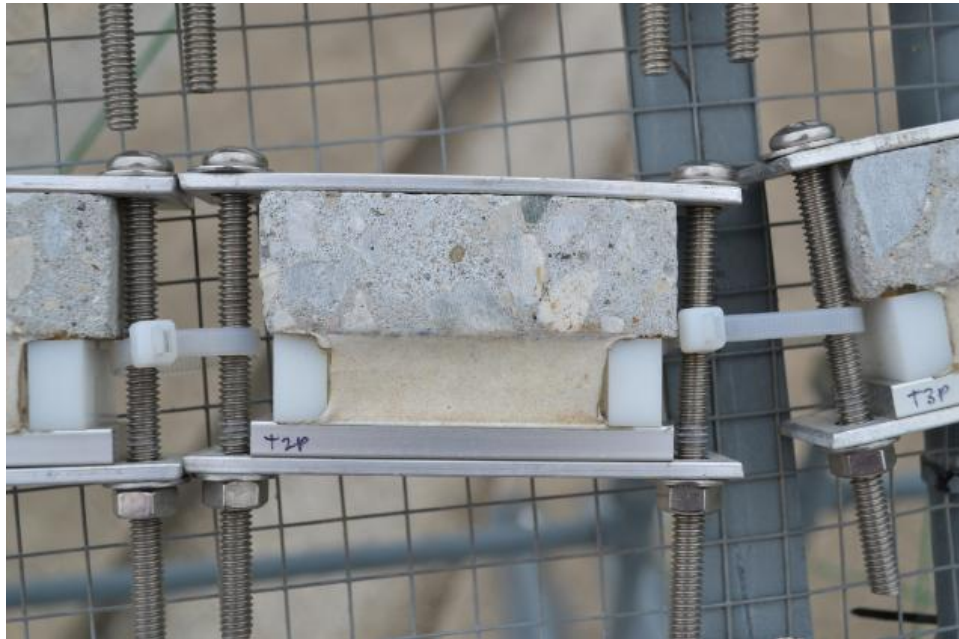
Figure 37: Sealant Specimen DRP1014-T2P (Silicone, SWRI Validated, Primed) Immediately After (top) and 4 Months in Extension (bottom)
