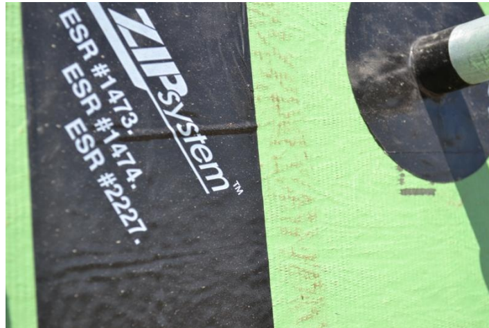
Figure 11: Fishmouthing of Specimen DRP1009-10 Tape at Sheathing Joint After 2 Months—4 Months Before Required Cladding
