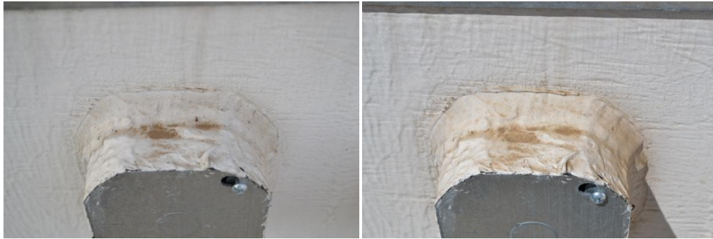
Figure 7: Dirtiness of Specimen DRP1009-11 After 4 Months (left) and After 1 Year and 3 Months (right)
