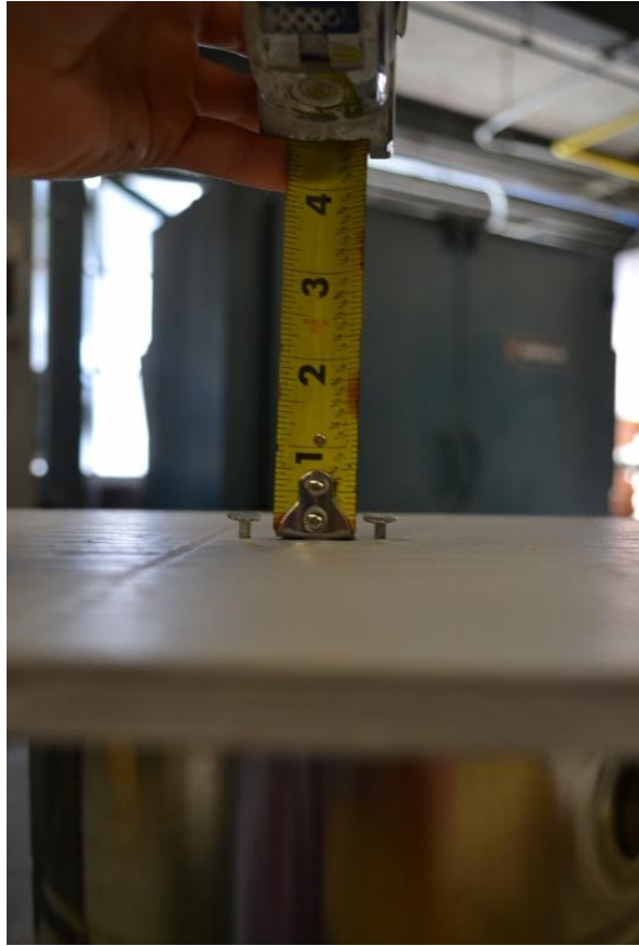
Figure 4: Nails Tapped Up \frac{1}{4} in. on Nail Sealability Specimen DRP1009-05-B
