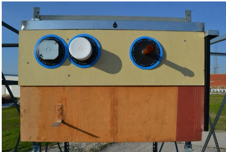
Figure 9: Specimen DRP1009-03 with Significant Discoloration 3 Months After Cladding
