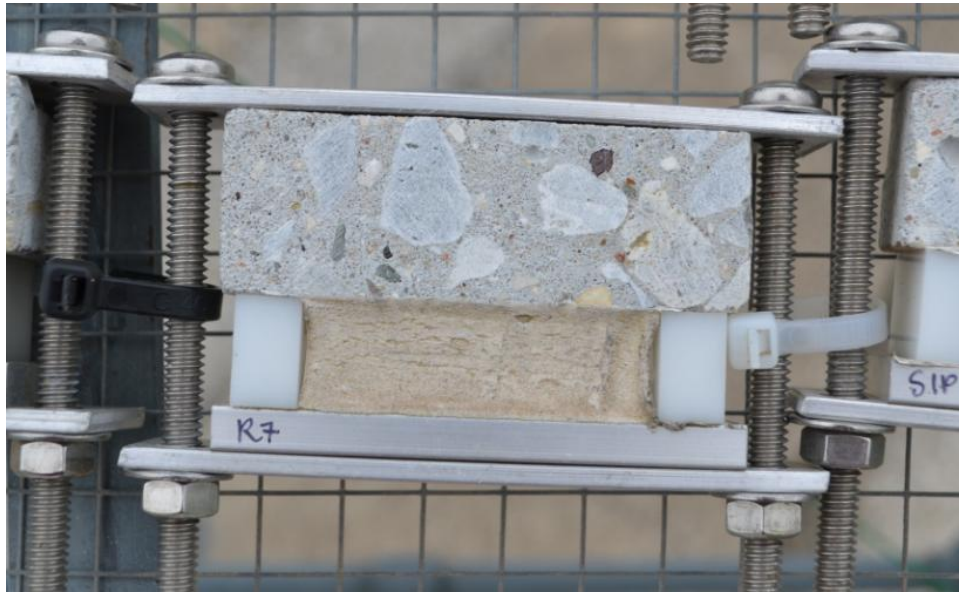
Figure 42. Specimen DRP1014-R7 Chain Scission After 4 Months in Extension
