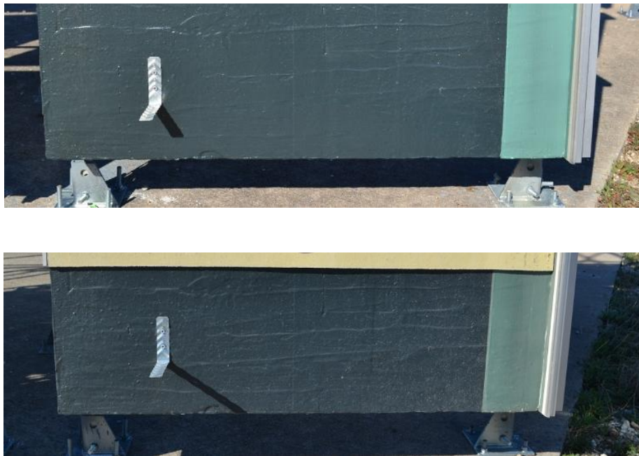
Figure 8: Dirtiness of Specimen DRP1009-07 at Installation (top) and After 1 Year and 3 Months (bottom)
