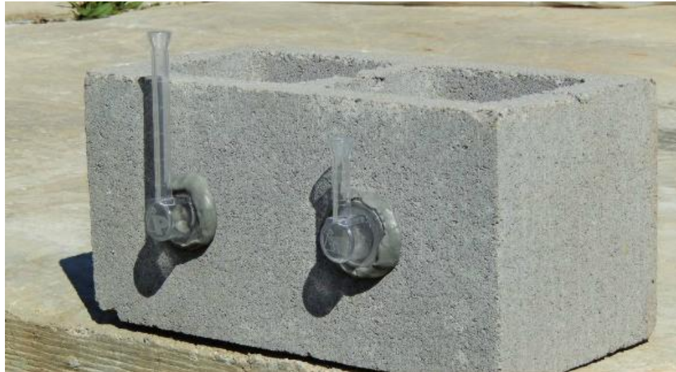
Figure 44: Tall RILEM tube (left) and Short RILEM Tube (right) (Chamra et al.)
