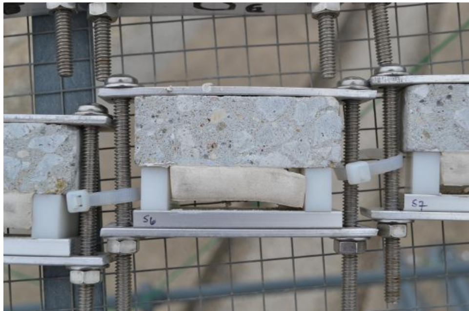
Figure 35: Sealant Specimen DRP1014-S6 (Urethane, Non-SWRI validated, Unprimed) Immediately After (top) and 4 Months in Extension (bottom)
