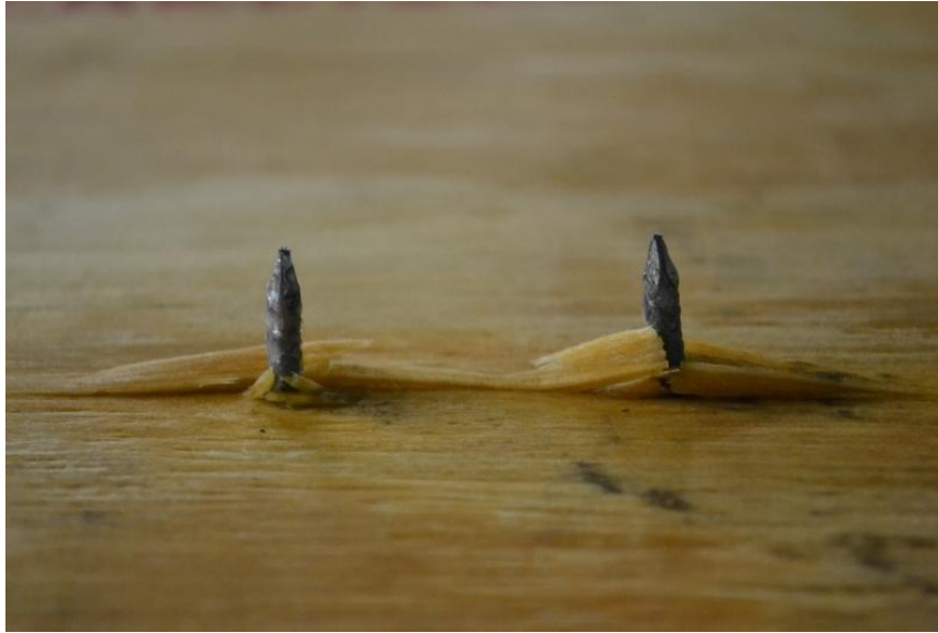
Figure 25: Visible Moisture Droplets on Nail Shanks of Specimen DRP1009-08-A
