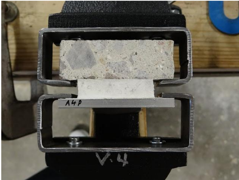
Figure 34: Specimen DRP1014-A4P in Metal Clamps of Vise Before Extension
