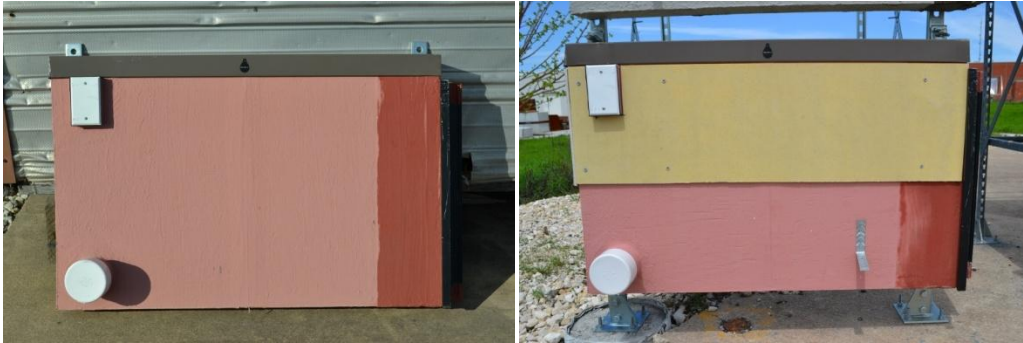
Figure 10: Specimen DRP1009-13 Comparison of Discoloration at 6 Months (left) and 1.5 Years (right)
