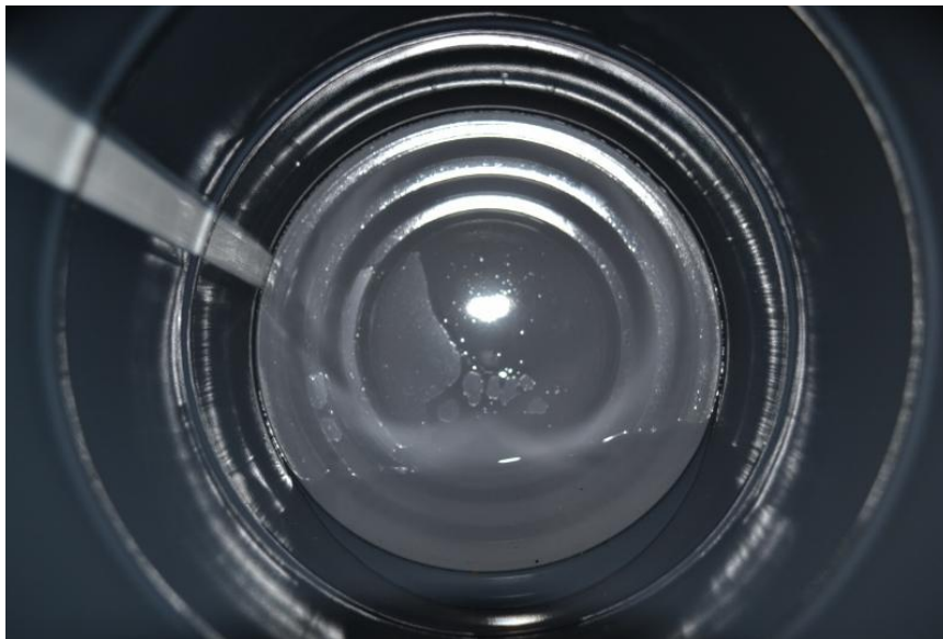
Figure 28: Water in Bottom Can of Specimen DRP1009-07-C
