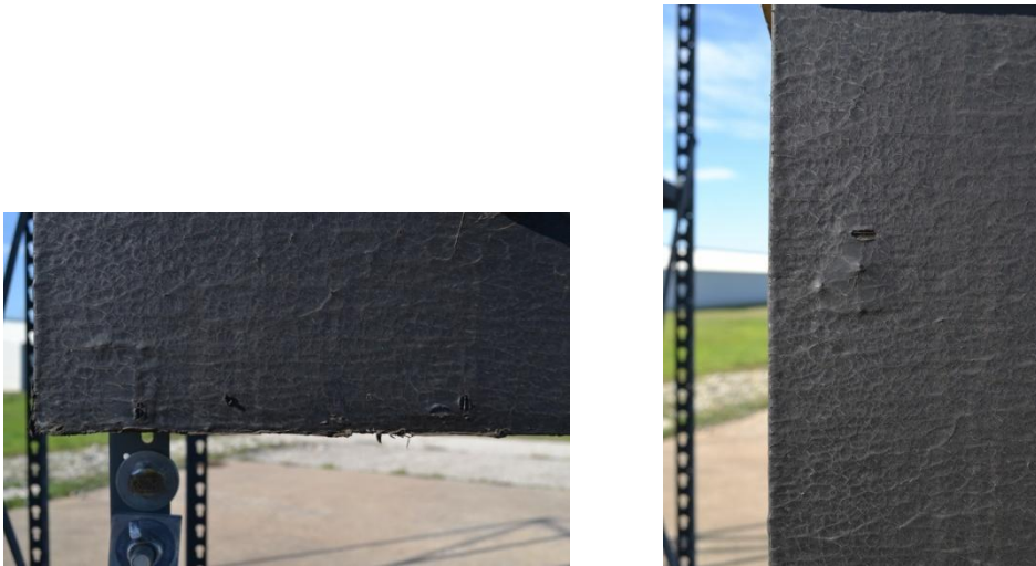
Figure 24: Specimen DRP1009-09 Blistering After 1 Year and 3 Months Exposure
