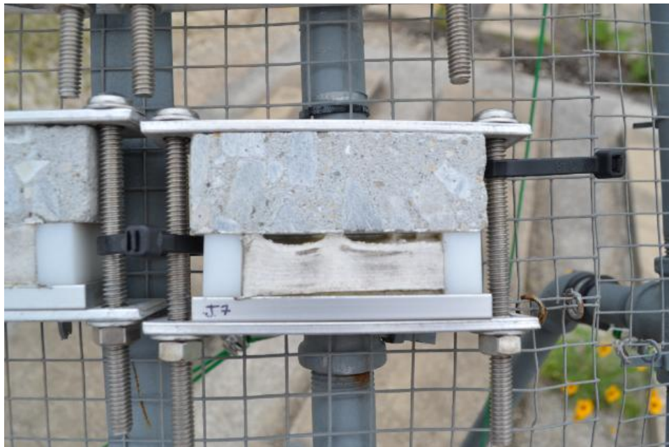
Figure 39: Sealant Specimen DRP1014-J7 (Urethane, SWRI Validated, Unprimed) Immediately After (top) and 4 Months in Extension (bottom)
