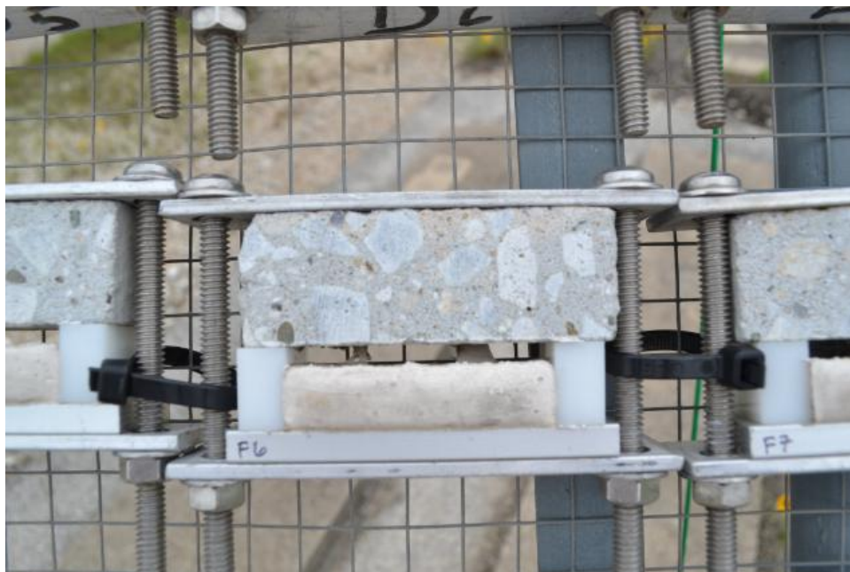
Figure 36: Sealant Specimen DRP1014-F6 (Urethane, Non-SWRI Validated, Unprimed) Immediately After (top) and Four 4 Months in Extension (bottom)
