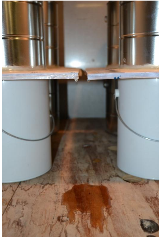
Figure 29: Water Leaking Out Corners of Specimen DRP1009-02-A and -B, Which are Wrap WRBs, Within Minutes of Placement in Environmental Chamber
