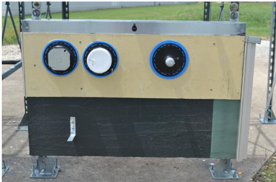
Figure 3: WRB Specimen DRP1009-07 Clad on Top Half
