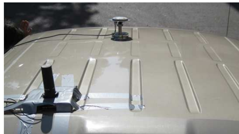
Fig. 6. Wardriving antennas placed on the roof of the vehicle.
