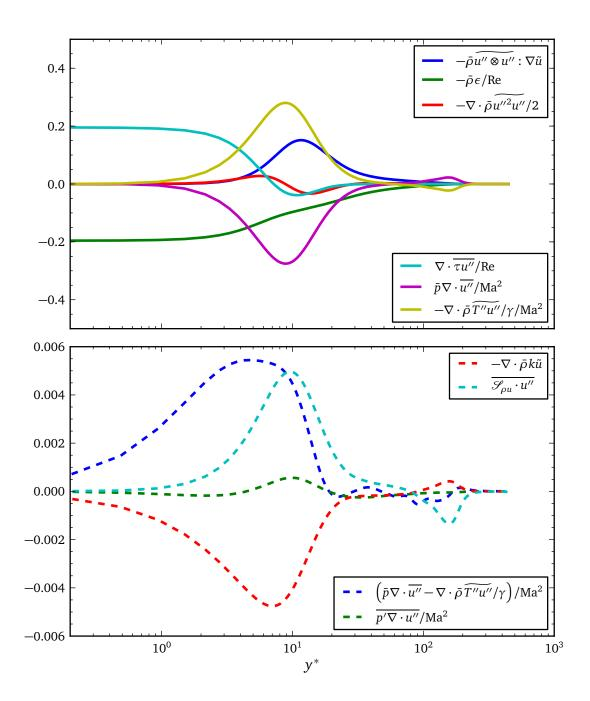
Figure 6.22: Budget for the turbulent kinetic energy (3.11d) in simulation t4.134 normalized by  $\rho_w u_\tau^4 / v_w$ . More significant terms appear in the upper half of the figure while less significant contributions appear in the lower half. Two nearly symmetric thermodynamic terms above have their sum duplicated below.
