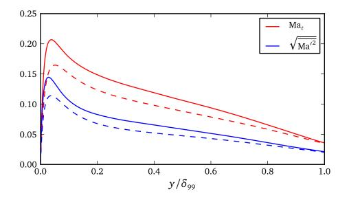
Figure 6.6: Turbulent Mach number  $Ma_t = \sqrt{2k}/\bar{a}$  and root-mean-squared local Mach number for simulations t3.199 (dashed) and t4.134 (solid).
