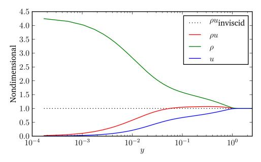
Figure 6.5: The inviscid base flow and viscous flow profiles for simulation t4.134
