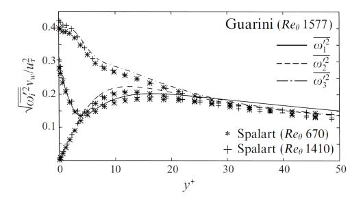
Figure 6.12: Root-mean-squared vorticity fluctuations from a Ma = 2.5, adiabatic-wall spatially homogenized boundary layer by Guarini et al. and incompressible results by Spalart [150]. Reproduced from Guarini et al. [60].
