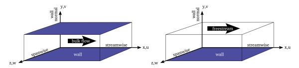
Figure 4.1: The channel (left) and flat plate (right) geometries.
