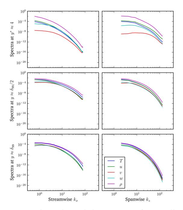
Figure 7.5: One-dimensional, unnormalized Fourier energy spectra from an ensemble over the location 2.299 m data appearing in Figure 7.4.
