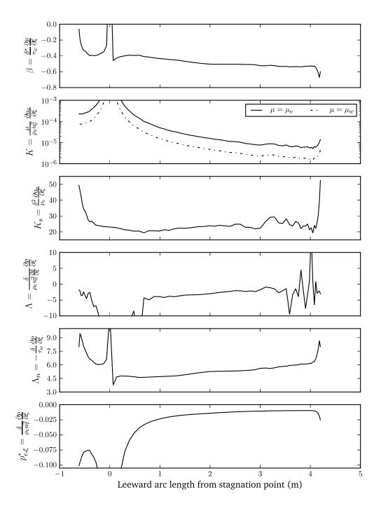
Figure 2.8: Pressure gradient conditions from the symmetry plane on a fully laminar Orion MPCV TPS simulation performed by P. T. Bauman.
