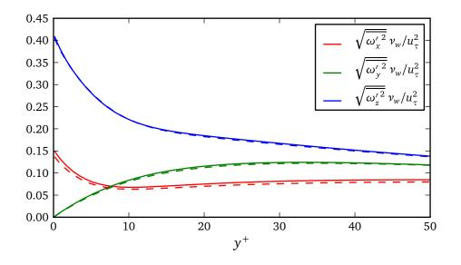
Figure 6.11: Root-mean-squared vorticity fluctuations normalized in wall units for simulations t3.199 (dashed) and t4.134 (solid).
