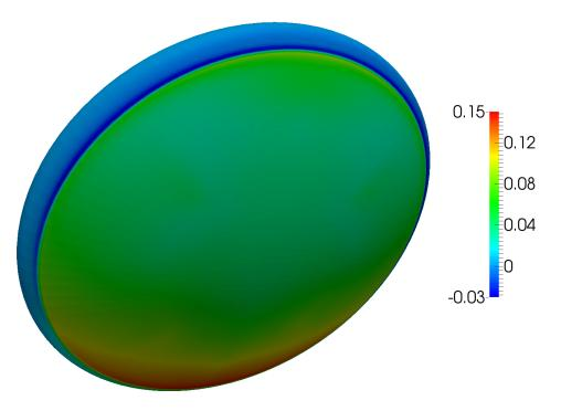
Figure 2.4: Normalized ablator recession rate difference between fully laminar and fully turbulent simulations,  $(\dot{m}_{turbulent} - \dot{m}_{laminar}) / \max(\dot{m}_{turbulent})$ , for Orion MPCV at peak heating conditions from International Space Station return trajectory. Data, which includes aerothermochemistry and ablation, courtesy of P. T. Bauman.
