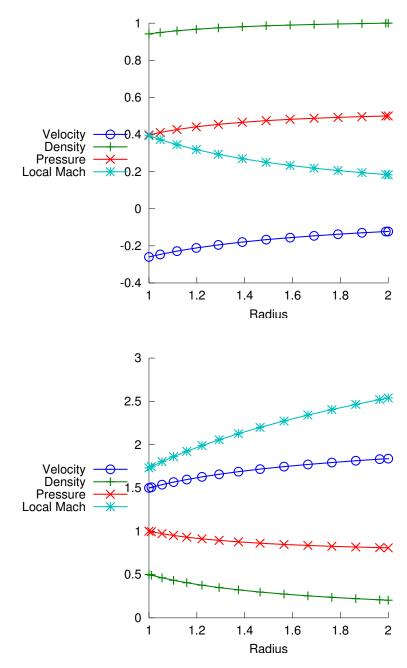
Figure C.1: Sample solutions saved by the radialflow.m demo logic in Listing C.1. The subsonic case (above) flows from right-to-left while the supersonic case (below) flows from left-to-right.
