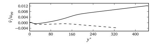
Figure 6.16: Mean wall-normal velocity normalized by the streamwise edge velocity for simulations t3.199 (dashed) and t4.134 (solid).
