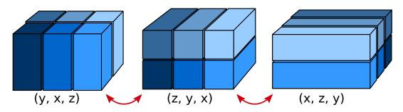
Figure 5.2: A pencil decomposition maps  $O(N^2)$  data to  $O(N^3)$  MPI ranks using two MPI\_Alltoall-like global communication phases depicted with red arrows. Each color represents the data owned by a single rank in each configuration.
