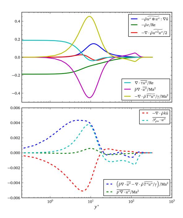
Figure 6.21: Budget for the turbulent kinetic energy (3.11d) in simulation t3.199 normalized by  $\rho_w u_\tau^4 / v_w$ . More significant terms appear in the upper half of the figure while less significant contributions appear in the lower half. Two nearly symmetric thermodynamic terms above have their sum duplicated below.
