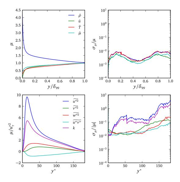
Figure 6.10: Reynolds-averaged primitive profiles (upper left) and Favre-averaged Reynolds stresses (lower left) with estimated standard errors as a fraction of mean (upper right, lower right) for simulation t4.134.
