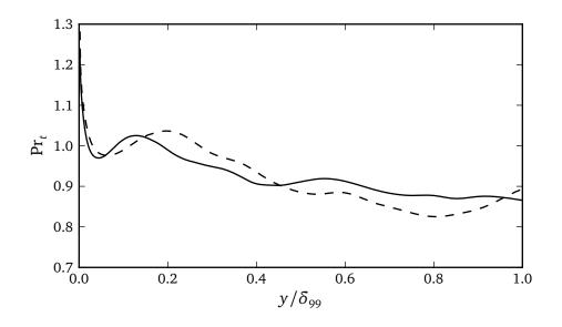
Figure 6.14: Turbulent Prandtl number  $\Pr_t = \frac{\widetilde{u''v''}\partial_y \tilde{T}}{\widetilde{T''v''}\partial_y \tilde{u}}$  for simulations t3.199 (dashed) and t4.134 (solid).
