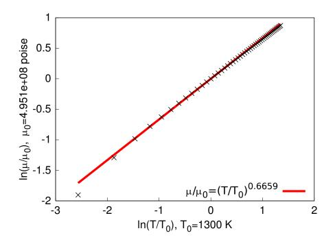
Figure A.1: Power law fit for air viscosity versus temperature over 100 to 5000 K using data from Svehla [157]. The least squares fit over this wide range is relatively insensitive to the chosen references  $\mu_0$  and  $T_0$ . For example, selecting  $T_0 = 300K$  or 4000K causes exponents 0.6639 or 0.6673 to be optimal, respectively. Truncating the data to eliminate larger *T* generally produces larger exponents.
