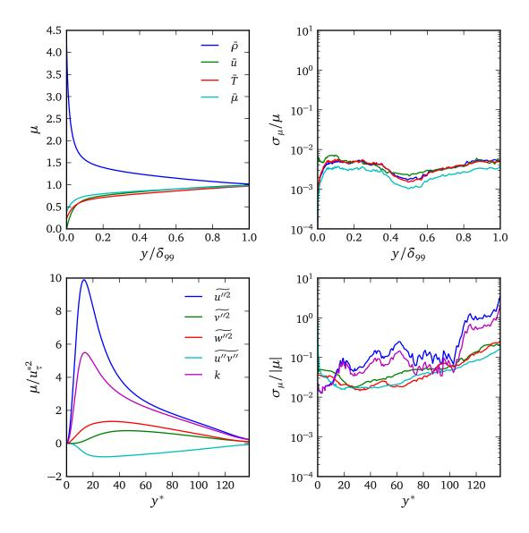
Figure 6.9: Reynolds-averaged primitive profiles (upper left) and Favre-averaged Reynolds stresses (lower left) with estimated standard errors as a fraction of mean (upper right, lower right) for simulation t3.199.
