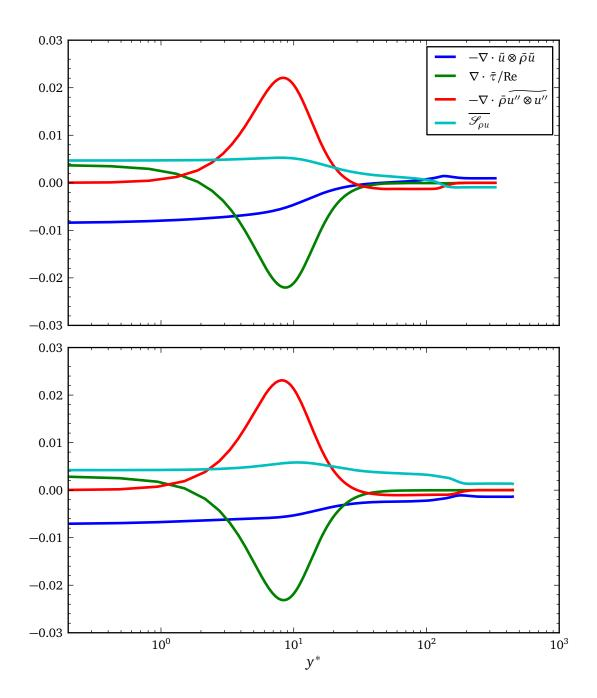
Figure 6.18: Budget for the Favre-averaged streamwise momentum (3.11b) in simulations t3.199 (above) and t4.134 (below) normalized by  $\rho_w u_\tau^3 / v_w$ .
