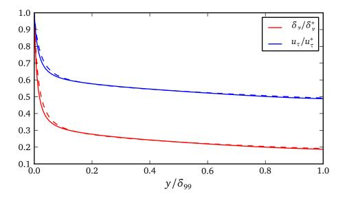
Figure 6.7: Comparison of viscous length and velocity scales using wall and semi-local units [67] in simulations t3.199 (dashed) and t4.134 (solid).
