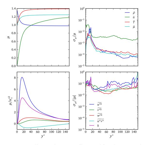
Figure 5.6: Reynolds-averaged primitive profiles (upper left) and Favre-averaged Reynolds stresses scaled by semi-local units [67] (lower left) with estimated standard errors as a fraction of mean (upper right, lower right) from simulation c03k15.
