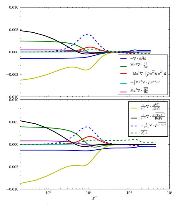
Figure 6.20: Budget for the Favre-averaged total energy (3.11c) in simulations t3.199 (above) and t4.134 (below) normalized by  $\rho_w a_w^2 u_\tau^2 / v_w$ .
