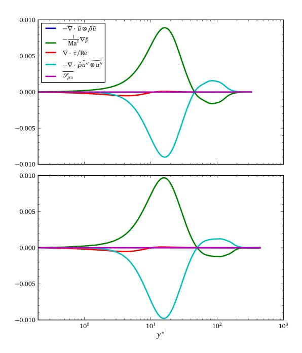
Figure 6.19: Budget for the Favre-averaged wall-normal momentum (3.11b) in simulations t3.199 (above) and t4.134 (below) normalized by  $\rho_w u_\tau^3 / v_w$ .
