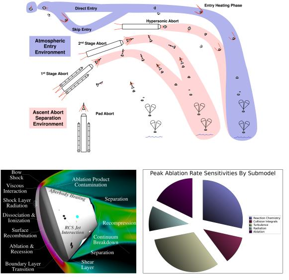
Figure 2.1: The Entry Heating Phase during atmospheric reentry is a complex multiphysics problem with uncertainties in system response predictions arising from many causes. In particular, aerothermodynamic heating and any associated ablative thermal protection system response predictions are highly sensitive to turbulence model parameters. Top and lower-left images courtesy of NASA. Lower right image reproduced from Stogner et al. [154].
