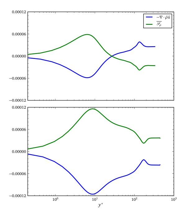
Figure 6.17: Budget for the Favre-averaged density (3.11a) in simulations t3.199 (above) and t4.134 (below) normalized by  $\rho_w u_\tau^2 / v_w$ .
