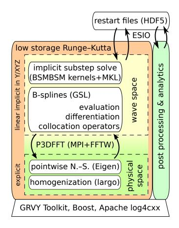
Figure 5.1: Architecture for the spectral simulation framework Suzerain
