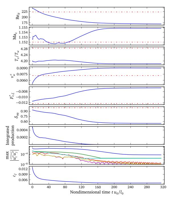
Figure 7.8: Fully turbulent initial condition study for location 4.314 m.
