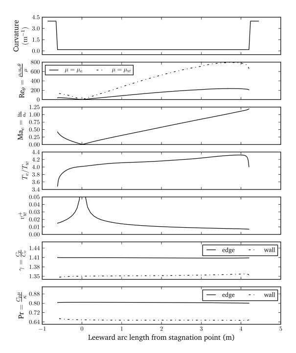
Figure 2.7: Reacting boundary layer conditions from the symmetry plane on a fully laminar Orion MPCV TPS simulation performed by P. T. Bauman.
