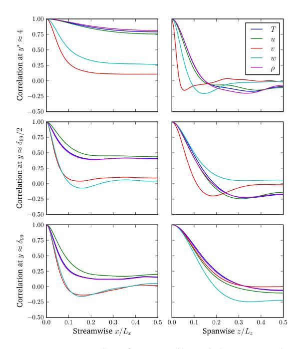
Figure 7.6: Two-point correlations from an ensemble over the location 2.299 m data appearing in Figure 7.4.
