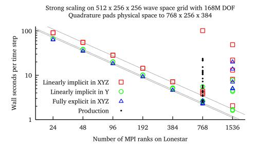
Figure 5.8: Strong scalability on a homogenized boundary layer scenario. At least three samples are present for each rank count and Navier–Stokes operator implementation. Workload is well-balanced at all rank counts. Grey lines indicate perfect parallel efficiency based upon 48-rank performance. Production timings, here implicit in only the wall-normal direction, included the overhead of writing statistics and checkpoint files.
