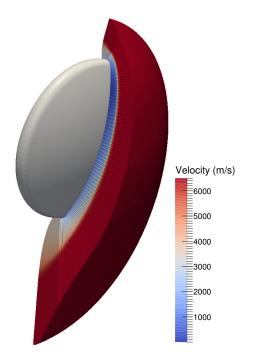
Figure 2.6: The velocity magnitude on the symmetry plane for a fully laminar Orion MPCV TPS simulation performed by P. T. Bauman.
