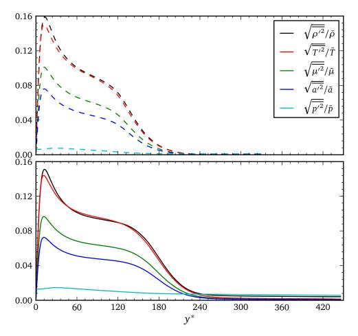
Figure 6.15: Root-mean-squared thermodynamic property fluctuations normalized by local means for simulations t3.199 (above, dashed) and t4.134 (below, solid).
