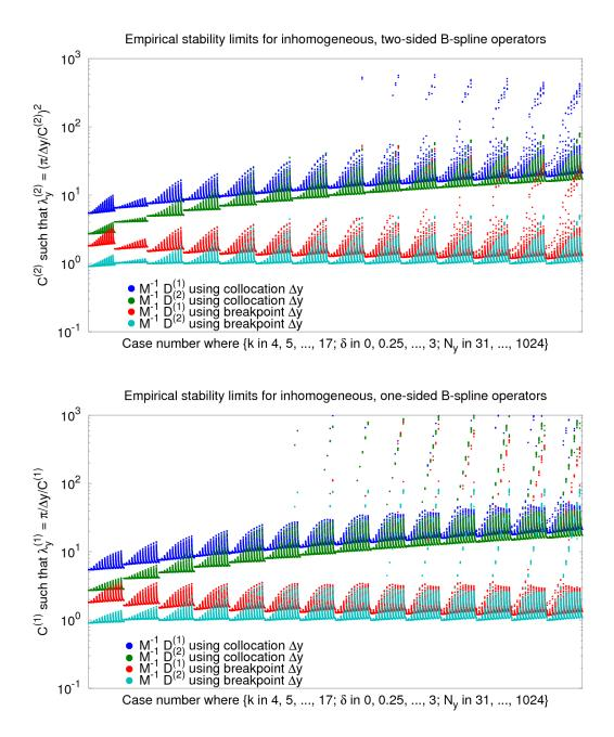
Figure 4.2: Exact values of  $C^{(1)}$  and  $C^{(2)}$  computed per Equations (4.17) and (4.20) for roughly 32,500 combinations of k,  $\delta$ , and  $N_y$ . Above, two-sided stretching was performed on breakpoints per (4.13). Below, one-sided stretching was performed per (4.14). In both figures, the leftmost four "triangles" correspond to k = 4 while  $\delta$  was varied slowly and  $N_y$  varied quickly. Moving rightward, the next "triangles" are for k = 5, then k = 6, etc.
