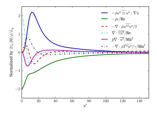
Figure 5.7: Budgets for the turbulent kinetic energy (3.11d) for channel simulation c03k15 normalized as by Huang et al. [67, figure 16a]. Omitted terms relative to (3.11d) are a factor of 25 times smaller than maximum production. [60].
