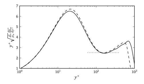
Figure 6.8: Examination of inner scaling in simulations t3.199 (dashed) and t4.134 (solid). For reference, the horizontal line shows  $1/\kappa$  for  $\kappa = 0.40$ .
